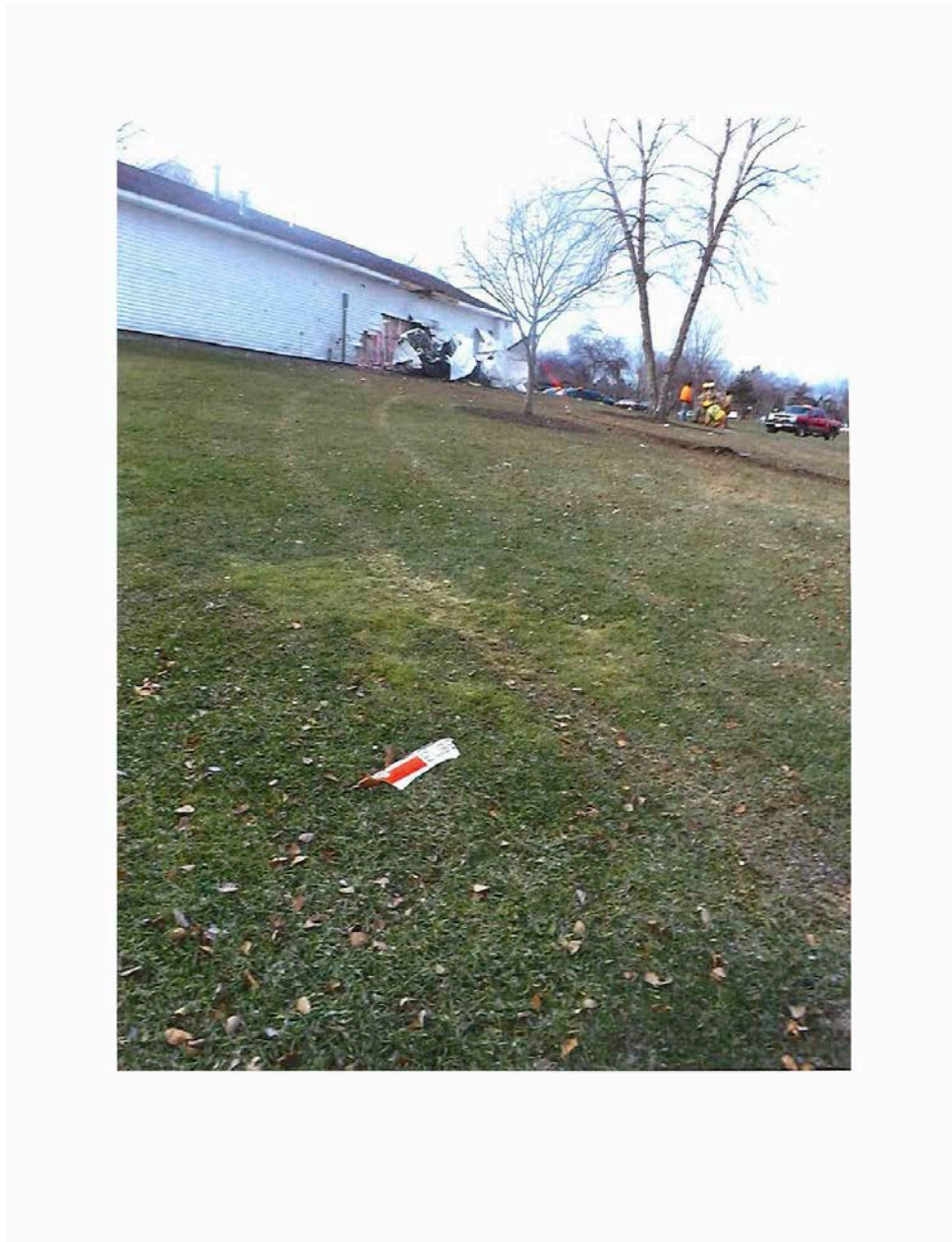
Photo 2 – Left wing tip separated when wing struck the ground.
