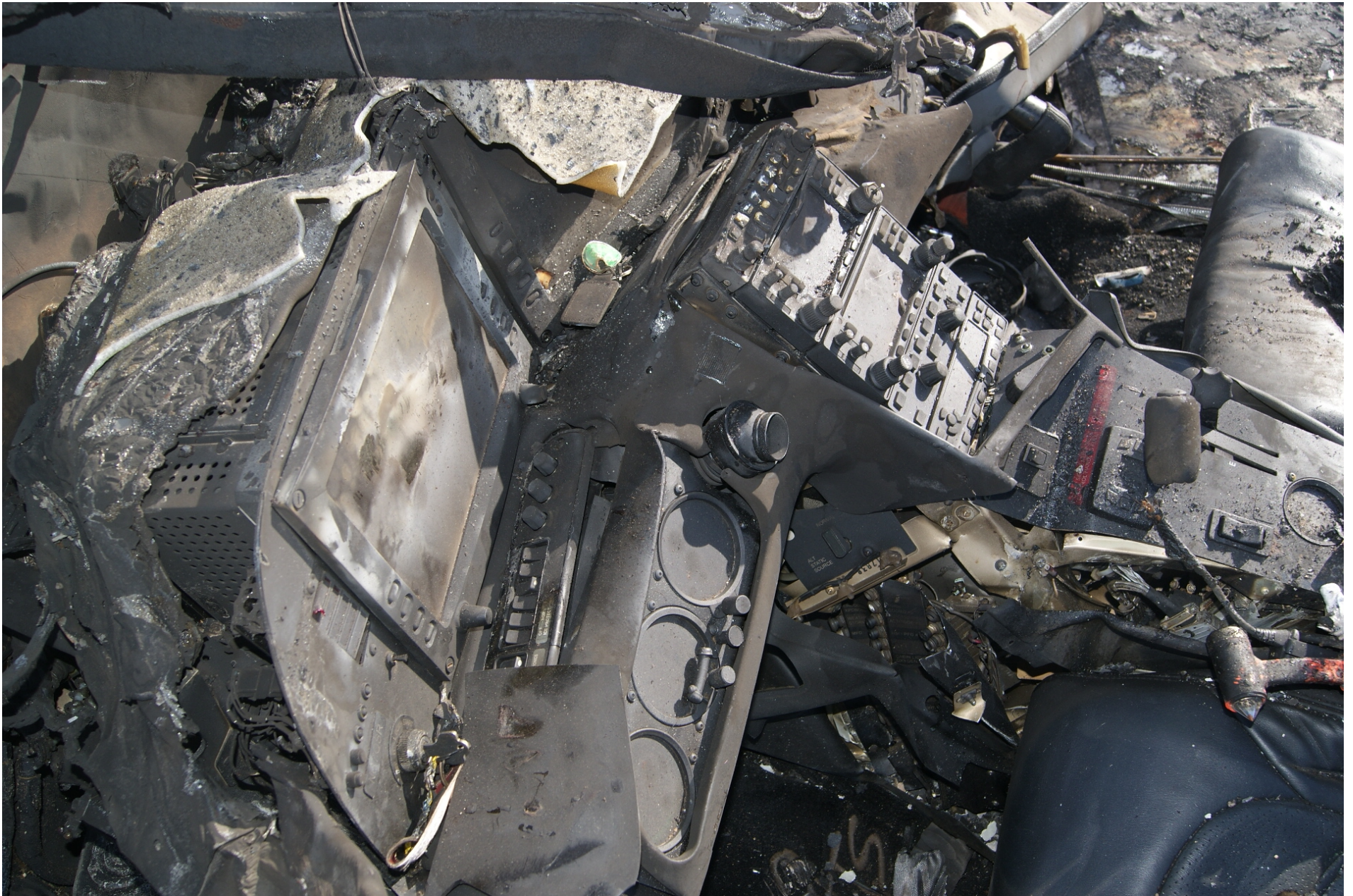
Photo 10 – The instrument panel. The PFD screen is in the center and the MFD screen is to its right.
