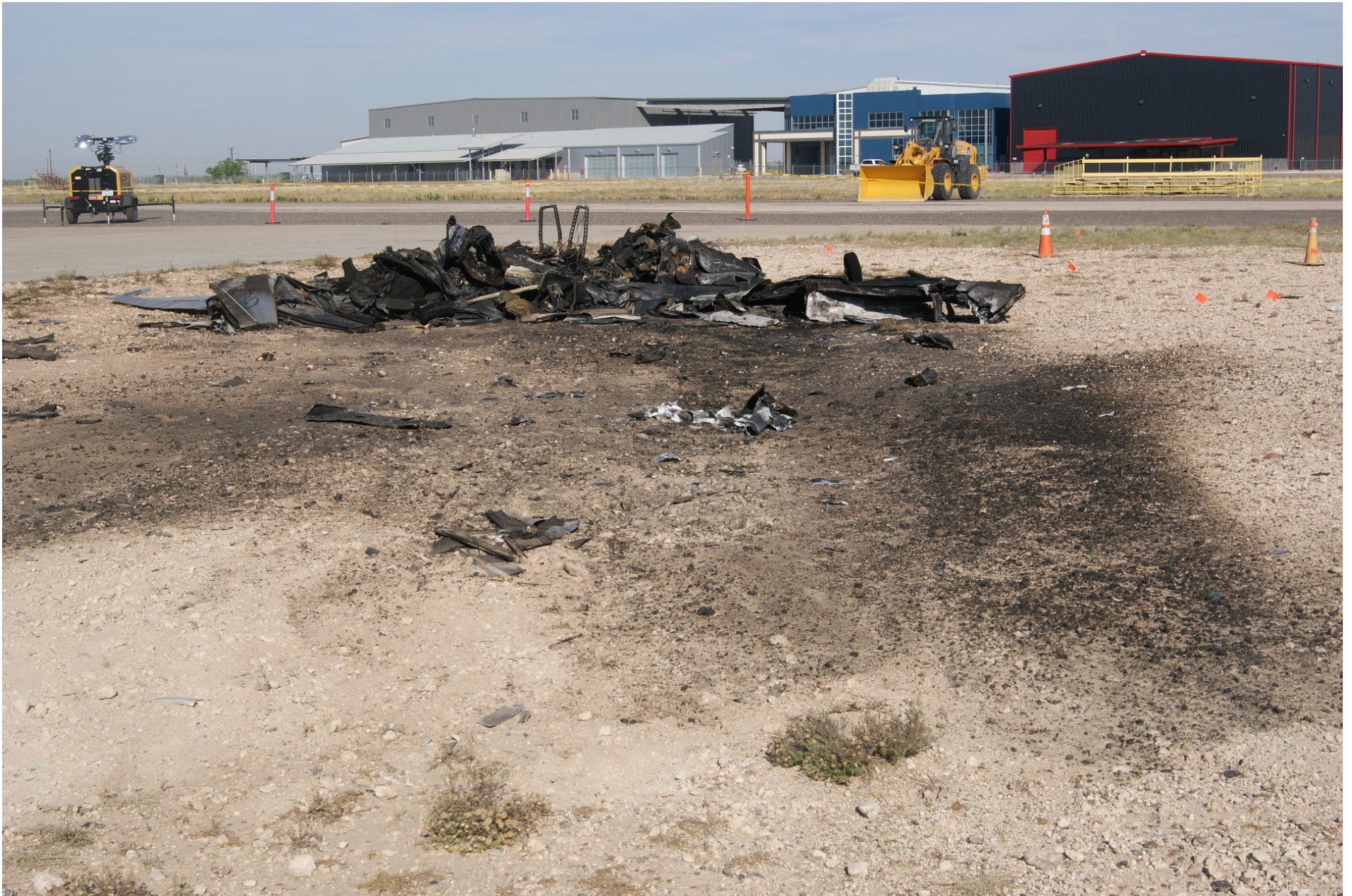
Photo 4 – The ground scar, leading to the wreckage, measured 53 feet in length and was aligned on a magnetic course of 270°.
