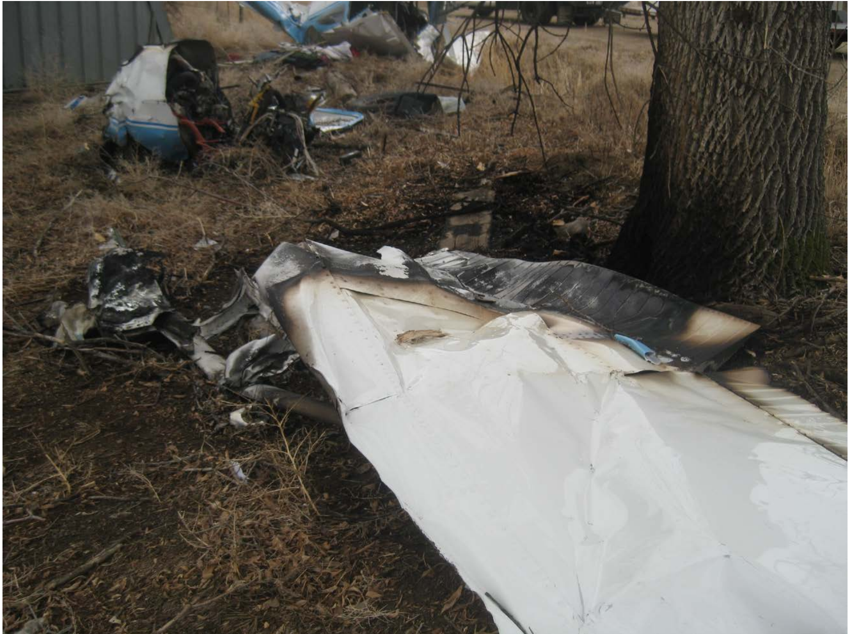
Photo 3 - Close-up view of severed right wing.
