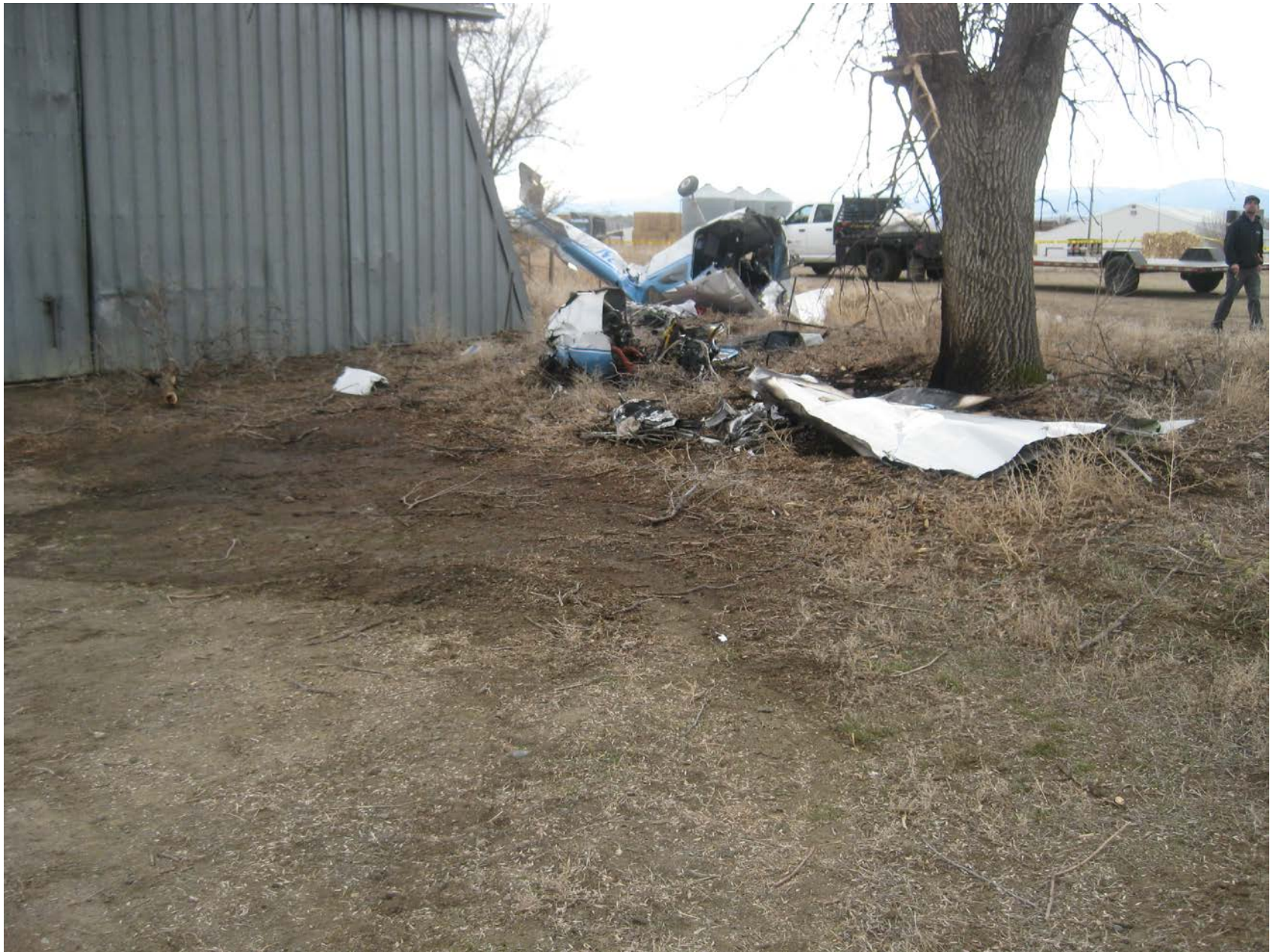
Photo 2 - N1095V at the crash site. Note burnt wing, grass, and tree trunk.
