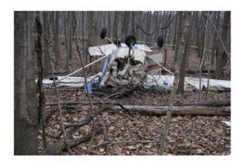
Photo 3 -Front of the airplane, exposing damage to the nose section and bottom of wings.
