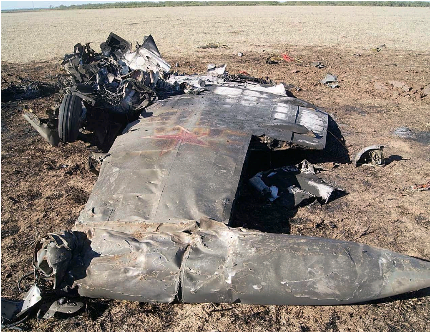
Photo 6 – Inverted right wing, remains of cockpit, and landing gear.
