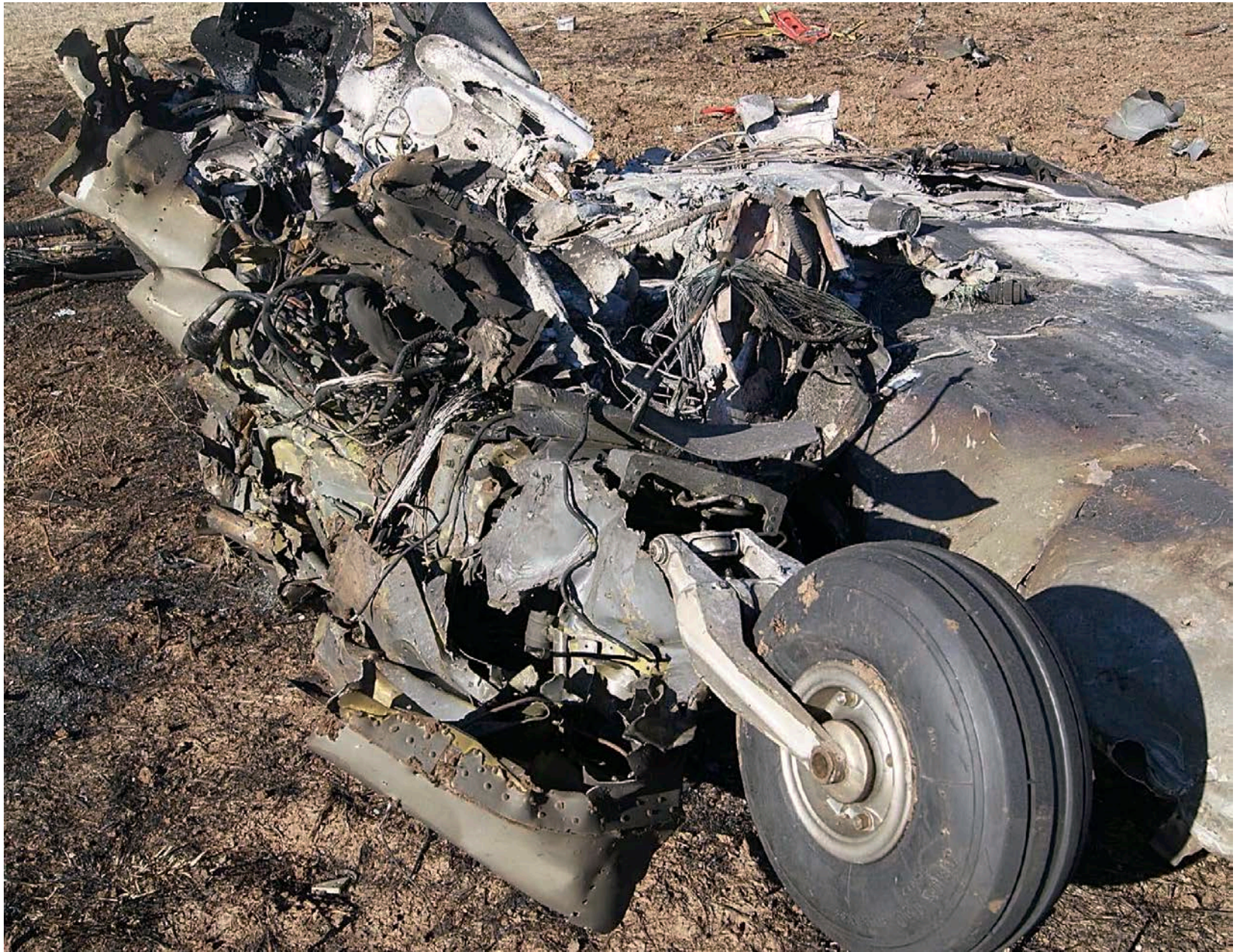
Photo 7 – Right main landing gear and portions of cockpit instruments.
