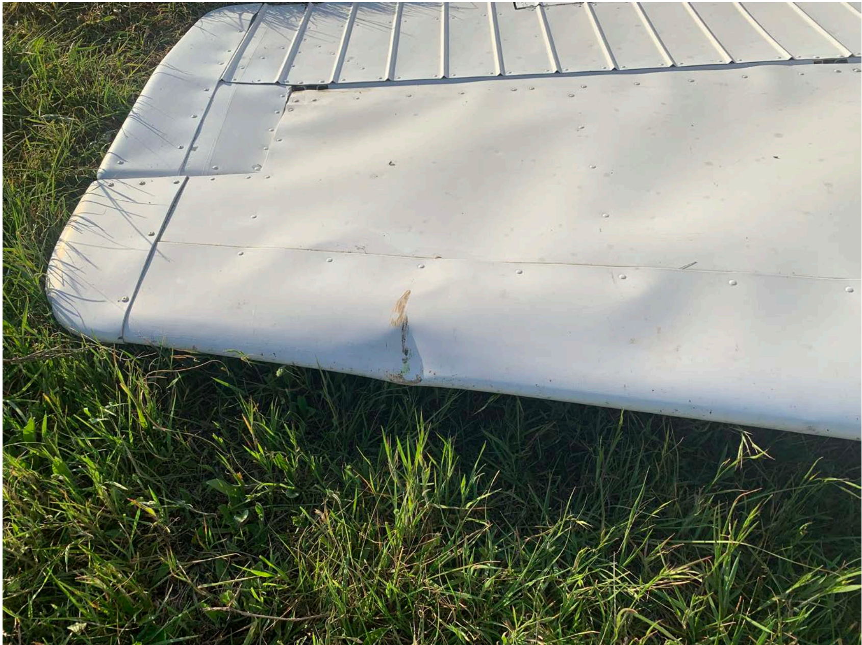
Photo 9 – Leading edge damage and skin wrinkles in right horizontal stabilizer (FAA photo)
