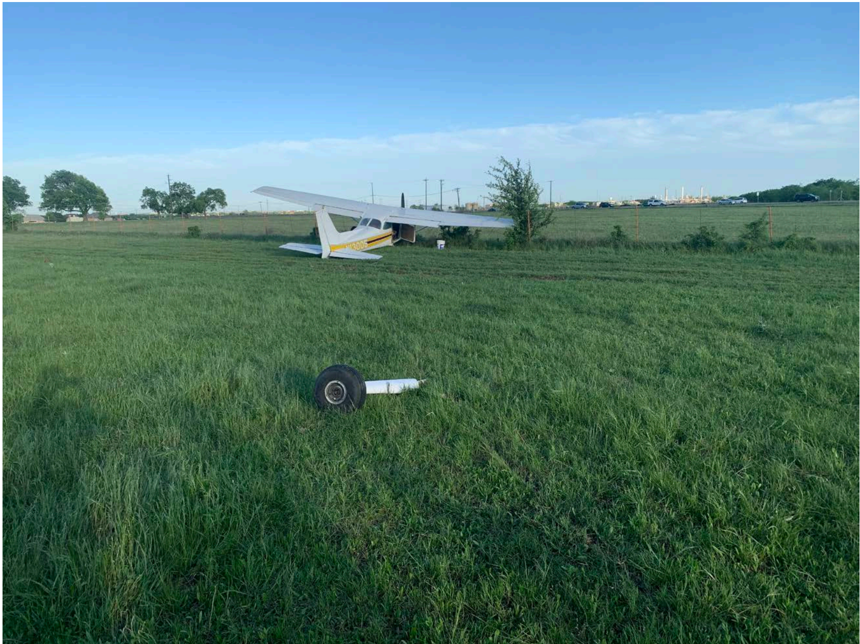
Photo 4 – N13005 sits against a second fence. Note severed right main landing gear in foreground (FAA photo)
