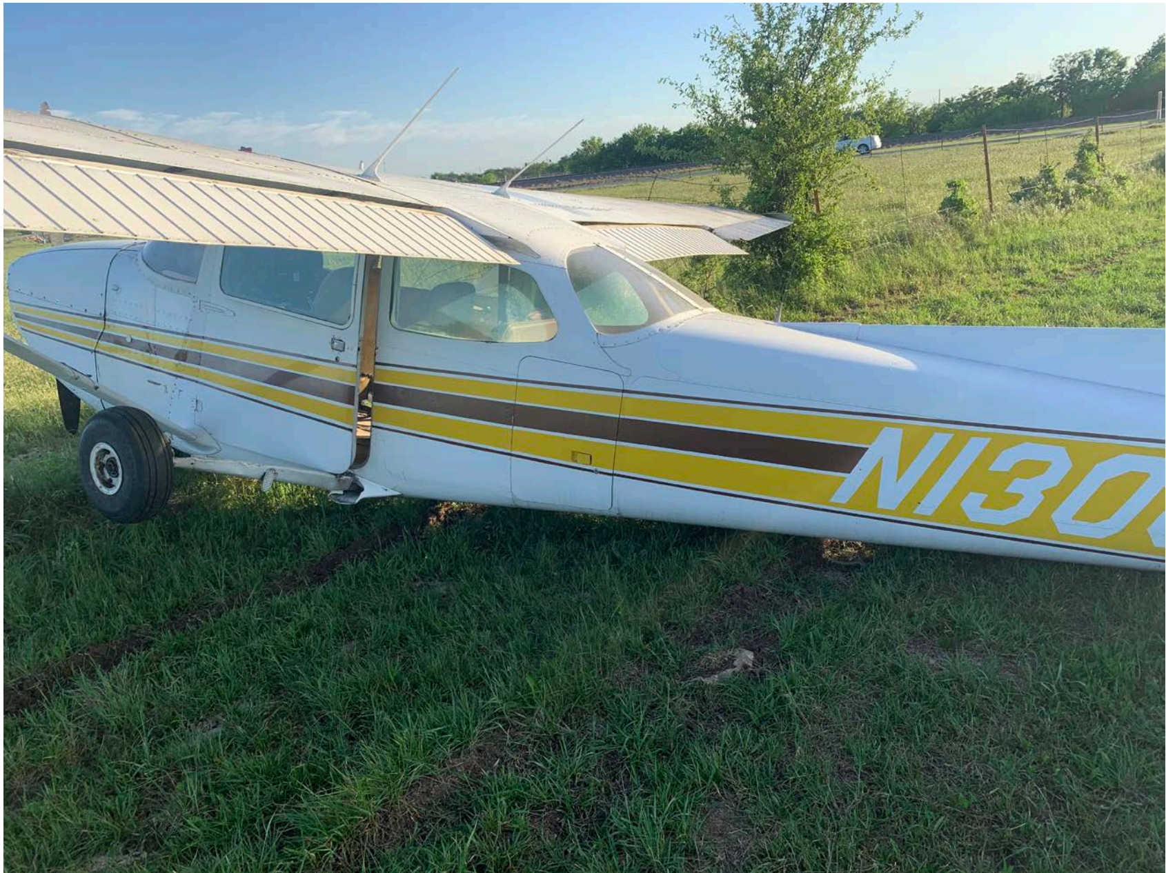
Photo 6 – Left main landing gear stayed attached but was bent forward (FAA photo)
