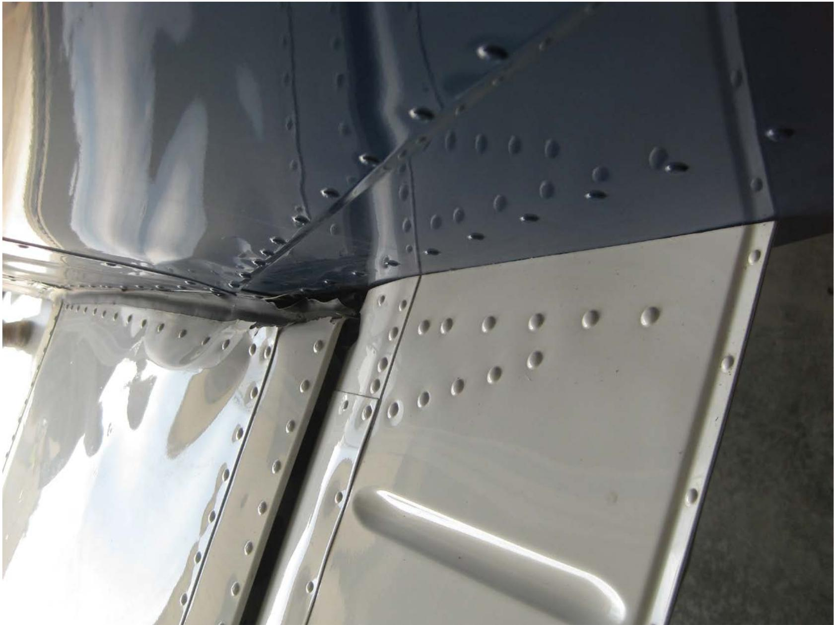
**Photo 7 – Torn skin on left wing and fuselage (FAA photo)**
