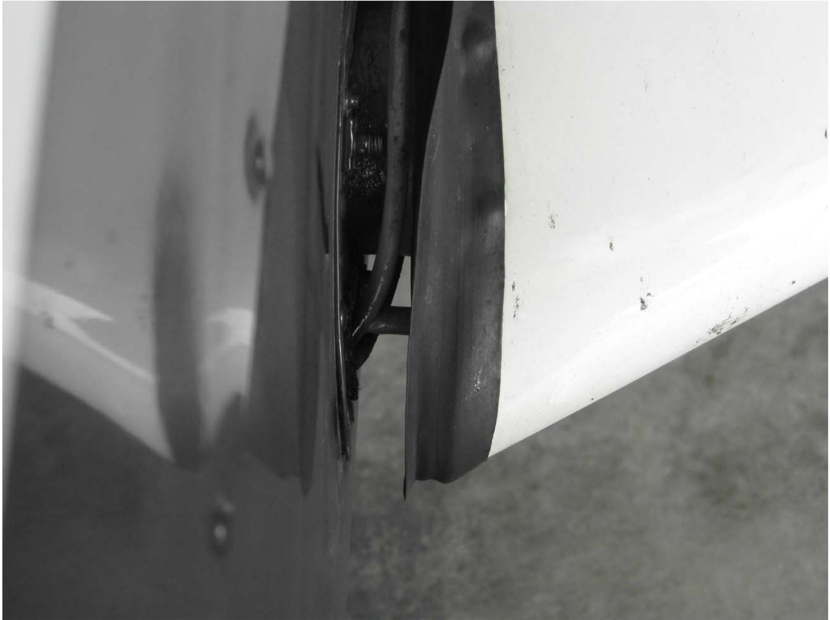
**Photo 4 – Left wing separation (FAA photo)**
