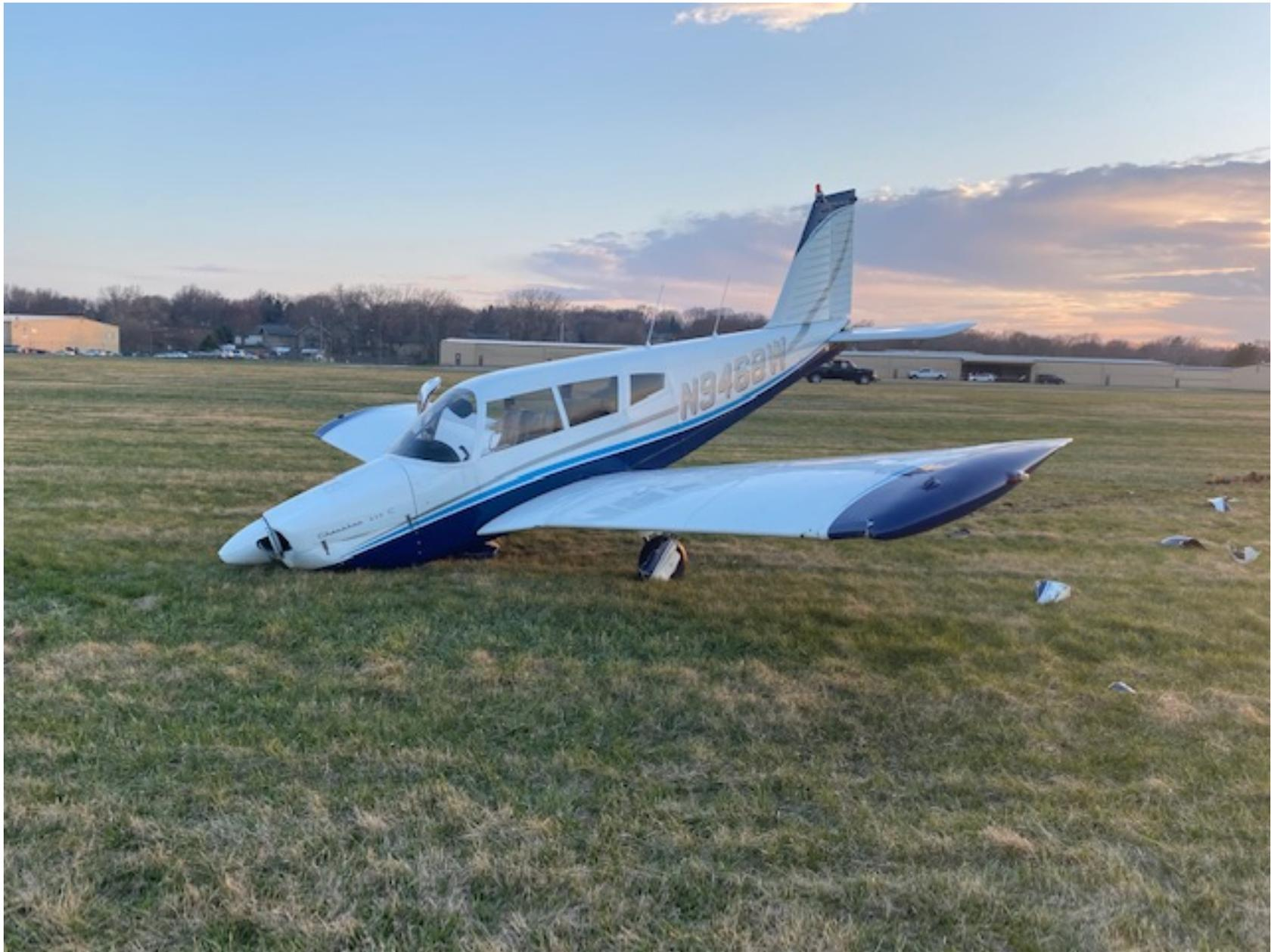
**Photo 3 – N9468W with collapsed nose landing gear (FAA photo)**
