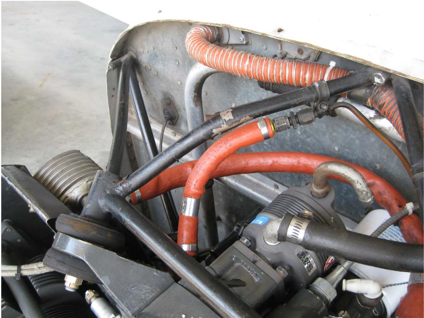
**Photo 5 – Bent engine mount and buckled firewall (FAA photo)**
