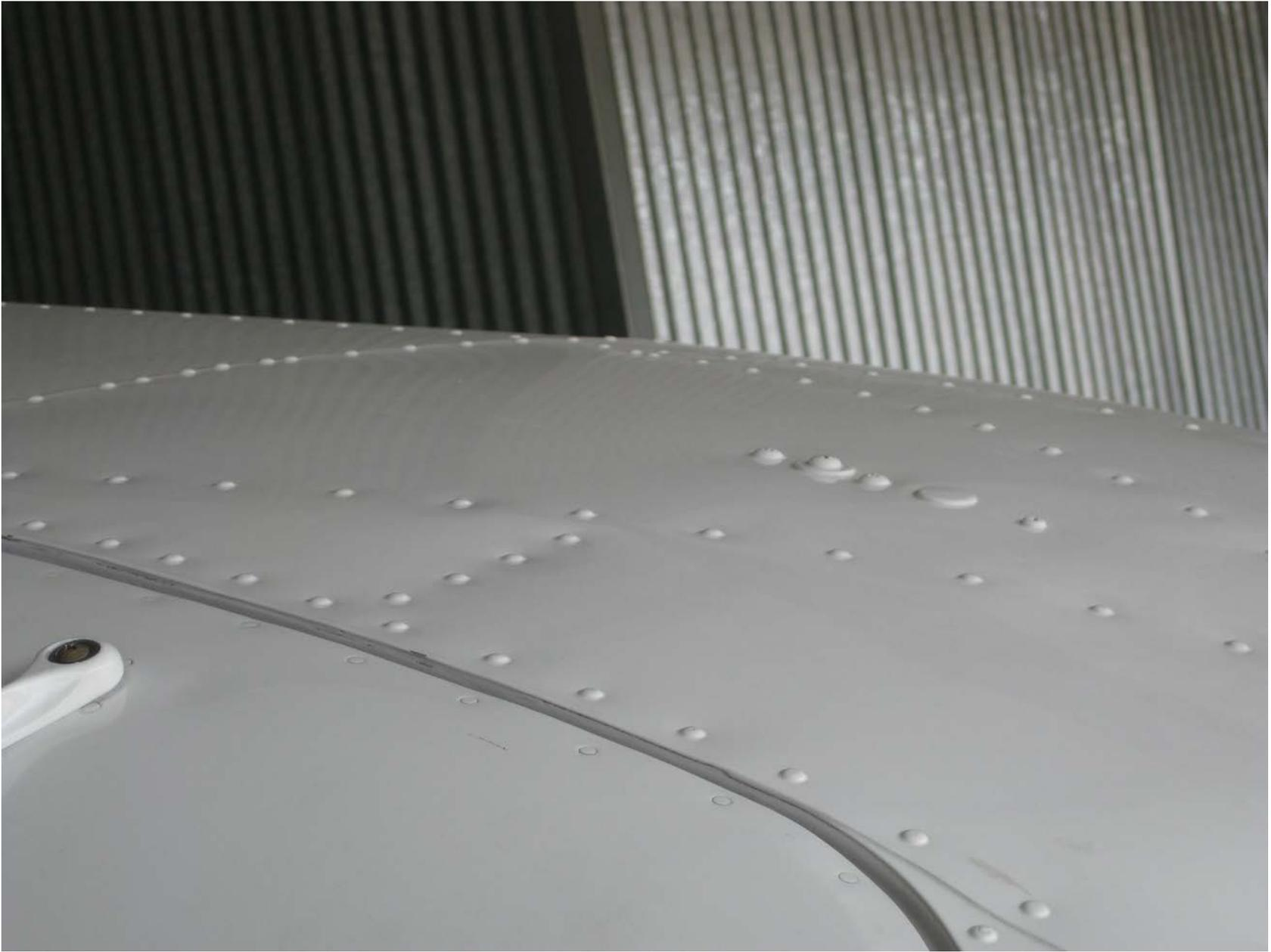
**Photo 6 – Wrinkle in roof next to cabin door handle (FAA photo)**
