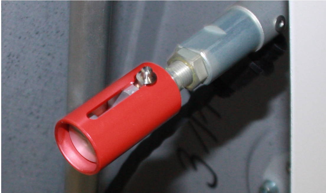
Figure 5a – secured quick-fastener, correct position of securing pin
