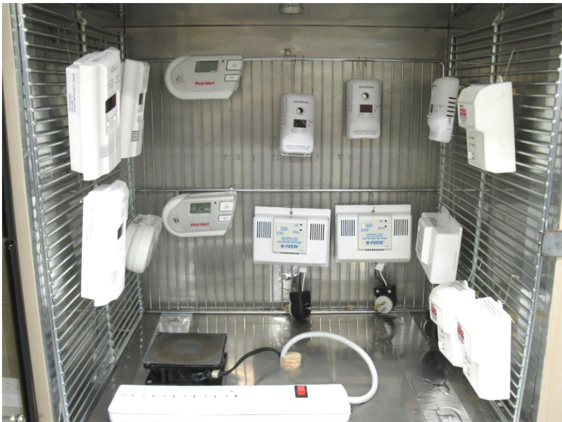
Various methane detectors undergoing testing in an environmental test chamber.
