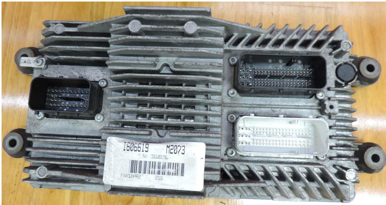
Figure 1. Front of International ECM removed from accident vehicle.
