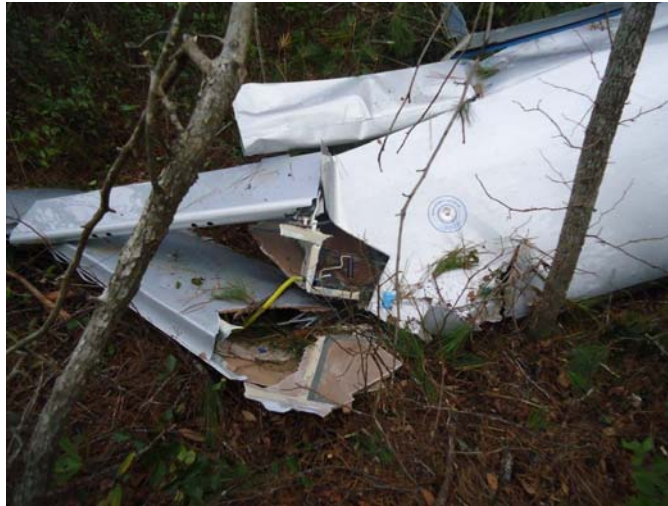
Figure 2: View of the Right Wing Fracture Location
