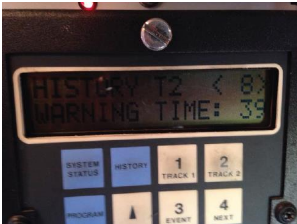
Figure-3 depicts warning time of the Grade Crossing Predictor to be 39 seconds
