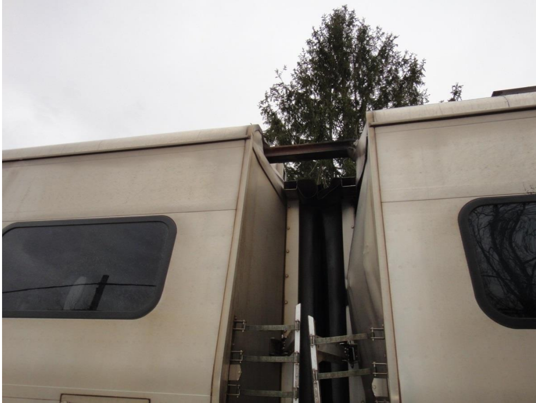
Figure 4- The third rail between the rear of car 4333 (on the right) and front end of car 4332
