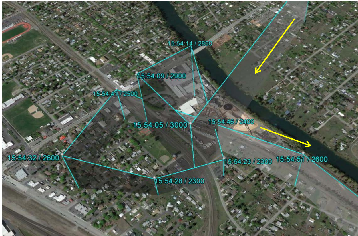
Figure 2. Aircraft flight path from GEG radar focusing on the sudden right turn after take-off. Yellow arrows indicate flight path.
