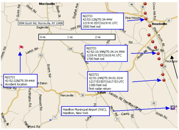
The suspected radar flight track of N22721, a Cessna 150H, is indicated by red dots.
