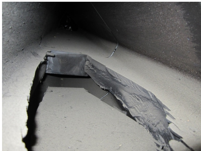
Photo 13- (b) (4) Fuel Grain Fracture
