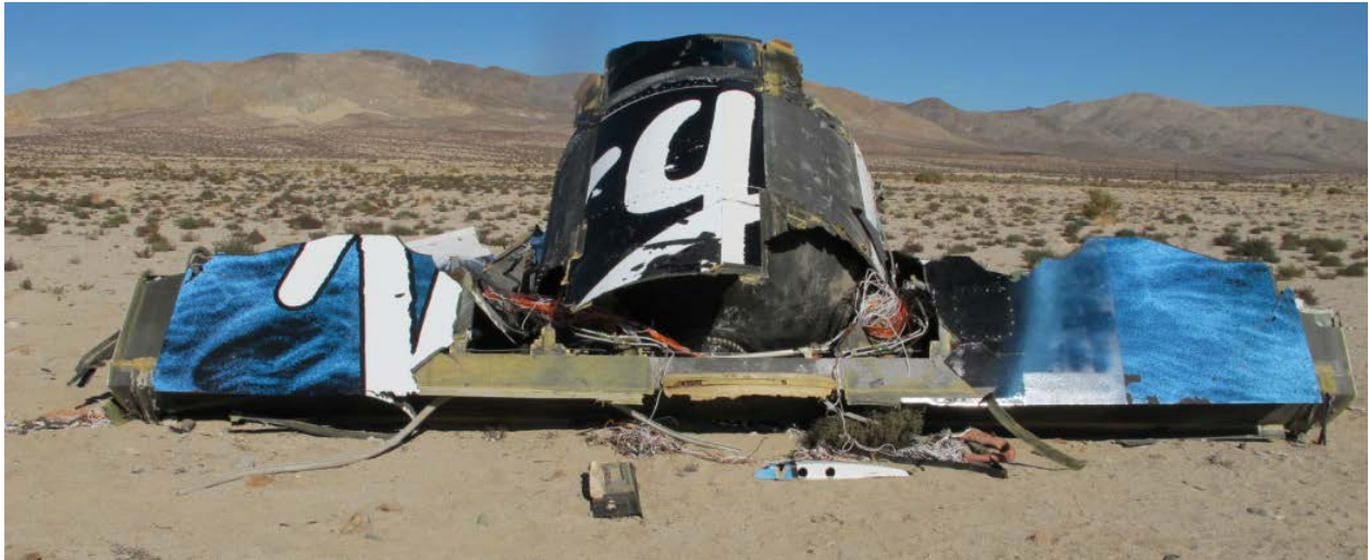
Photo 2- Fuselage Wreckage with Integral MOT, Inverted, Aft Side
