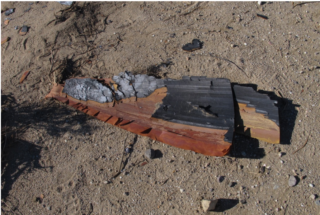
Photo 11- Rocket Nozzle Fragment Charring
