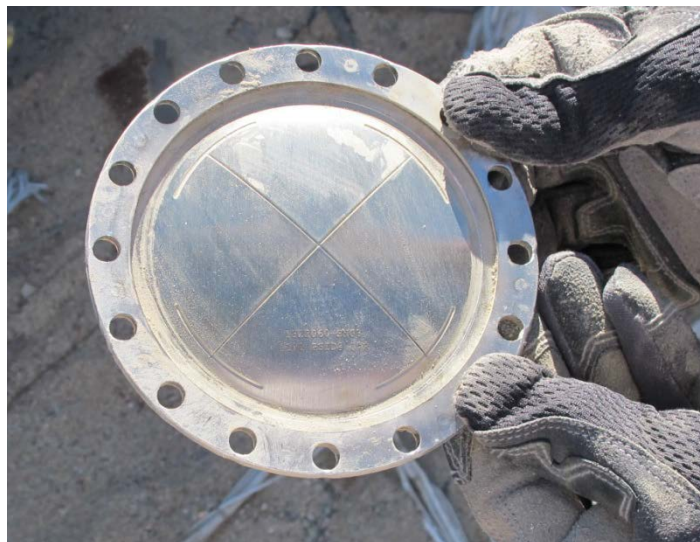
Photo 3- MOT Burst Disk, Intact
