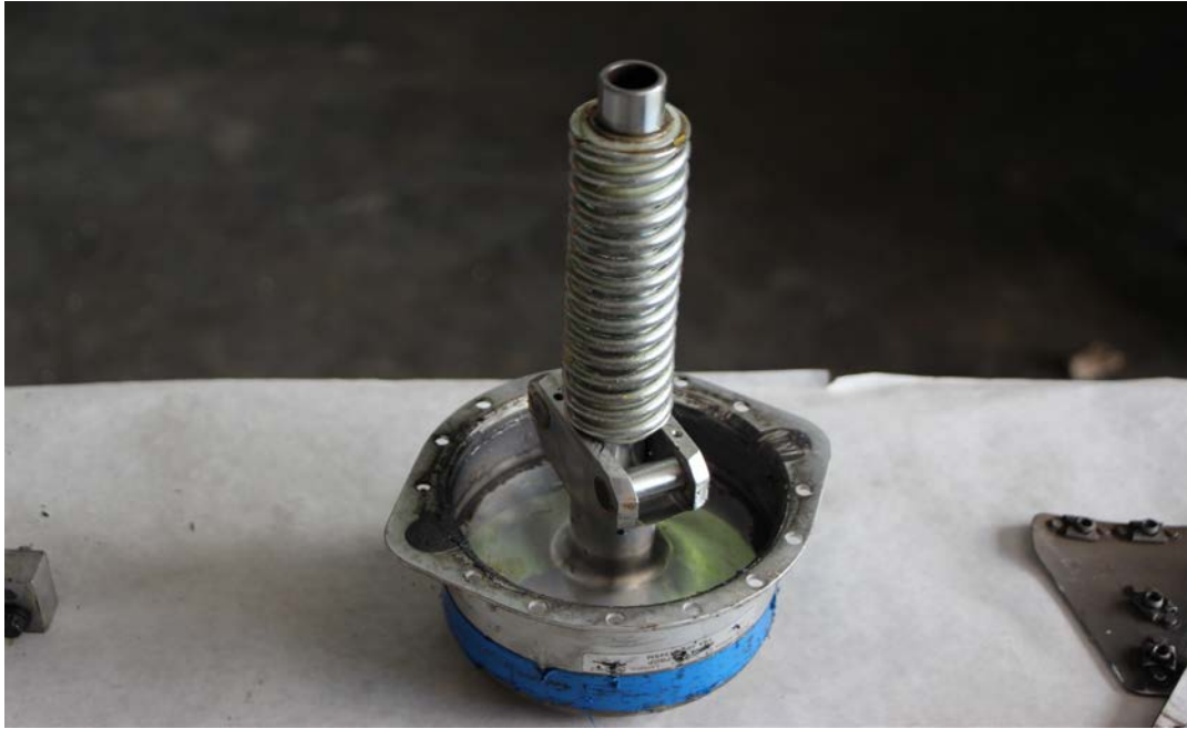
Photo: pitch change rod and spring.
