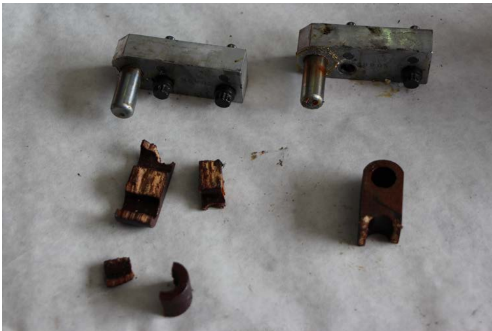
Photo: blade knobs, pitch change blocks
