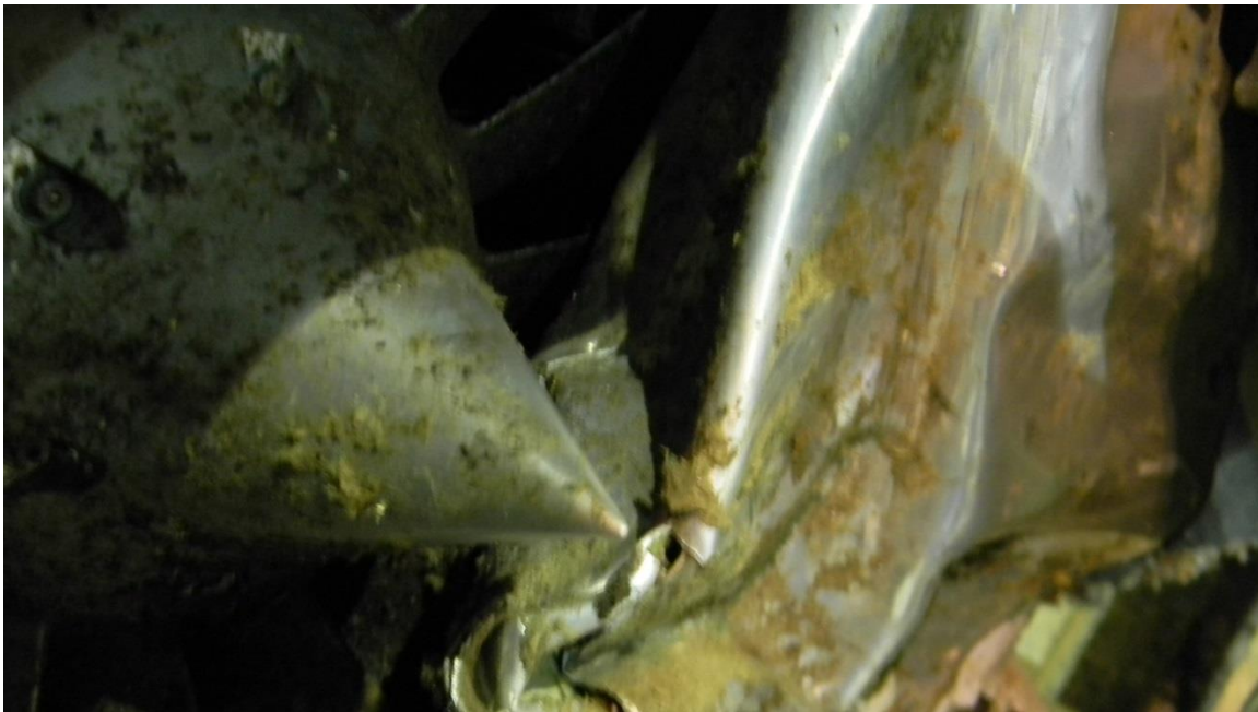
Figure 5- Right hand engine inlet, fan blades and spinner. Note debris deposited on fan blades, spinner and inlet, evidence consistent with no engine rotation during impact sequence.
