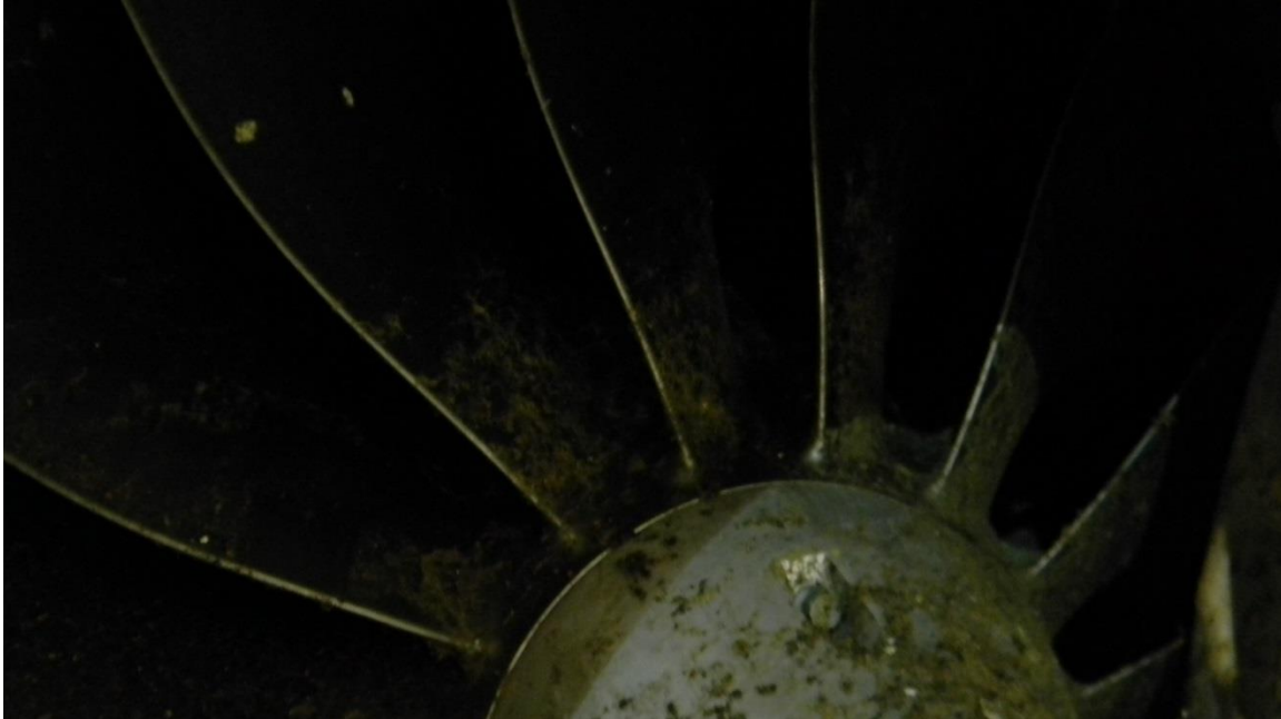
Figure 4 - Right hand engine fan blades and spinner. Note debris on fan blades and spinner, evidence consistent with no engine rotation during impact sequence.
