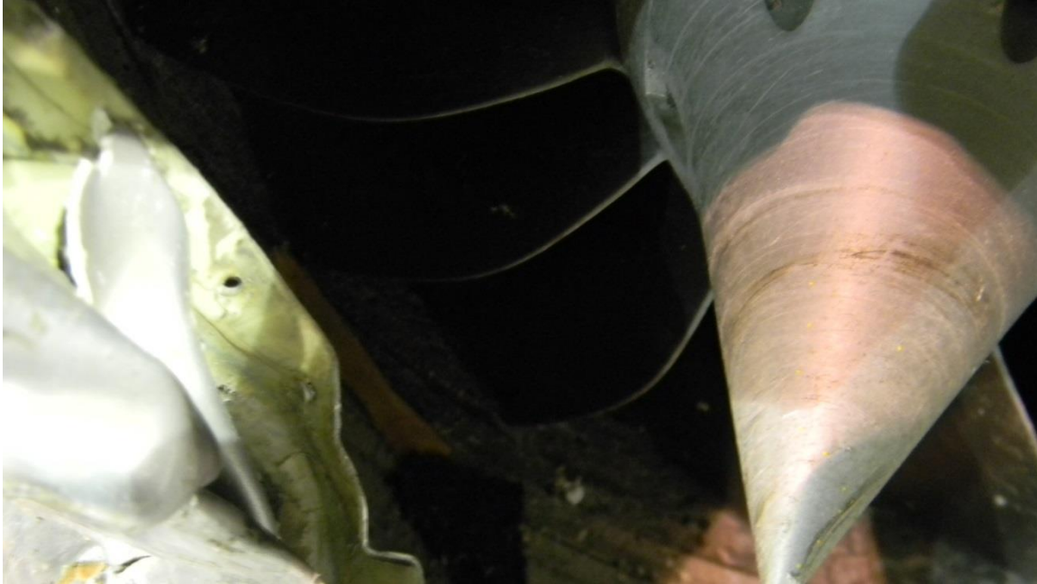
Figure 2 - Left Engine spinner and inlet. Note circumferential scratches on the spinner and lack of FOD, evidence consistent with engine rotation at impact.
