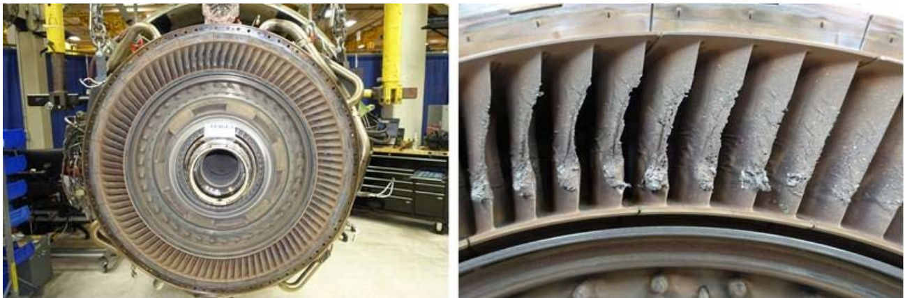
Photo 6- LPT S1 Nozzle Vane Trailing Edge, (R) Close up at 12 o'clock
