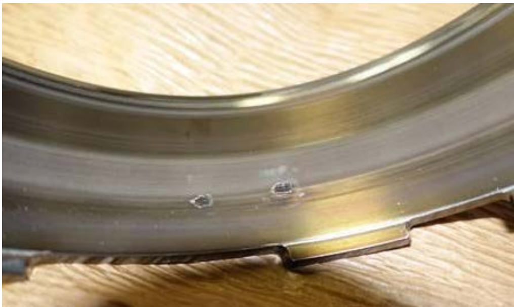
Photo 10- No. 4 Bearing Outer Race Debris
