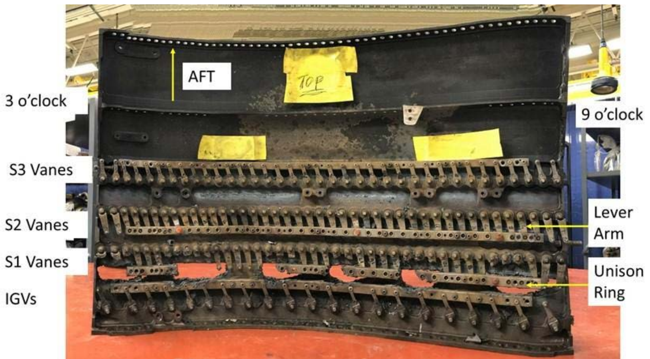
Photo 15- Panoramic Photo of HPC Stator Case (Exterior), Top Half
