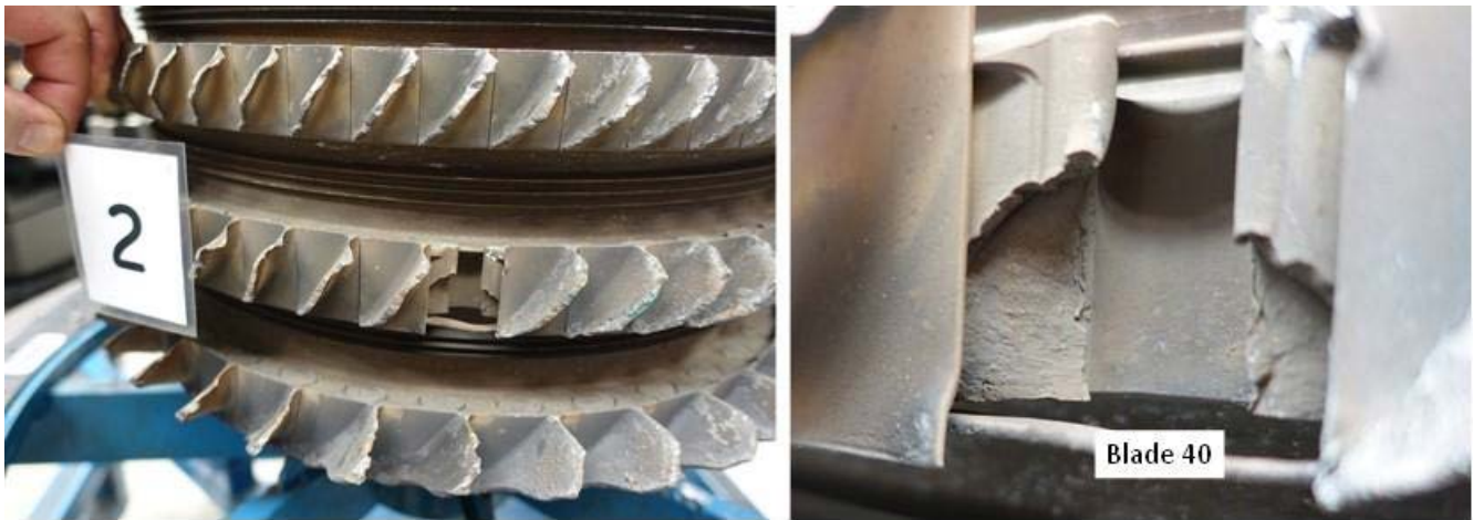
Photo 20- HPC S2 Missing Blade 40, Fractured Disk Posts
