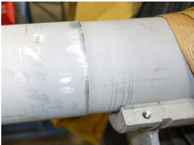
Photo 8- (L) LPT Shaft Rub, (R) LPT Shaft Light Impact Marks
