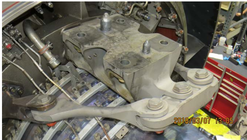
Photo No. 52: View of forward engine mount. (P&W)
