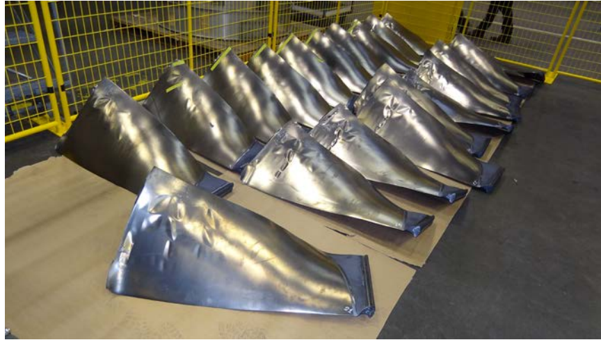
Photo No. 36: View of other fan blades after that had been removed from the engine. (Boeing)
