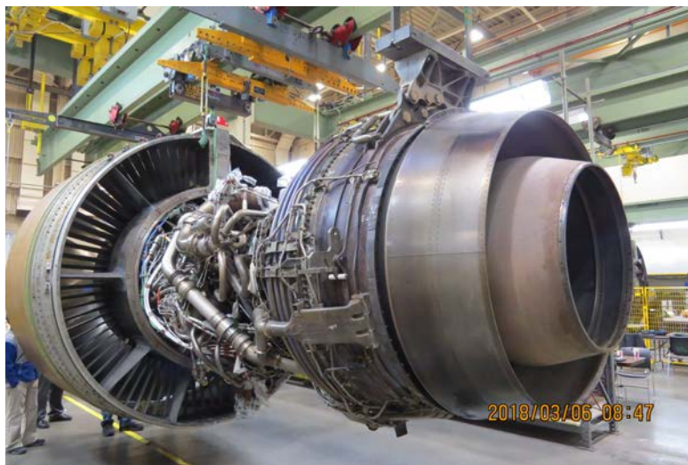
Photo No. 21: View of left side of engine showing no indications of an uncontainment, case rupture, or fire. (P&W)
