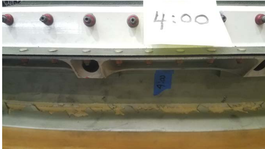
Photo No. 26: View of front of forward edge of Kevlar wrap showing chipped paint and aft movement of wrap. (P&W)
