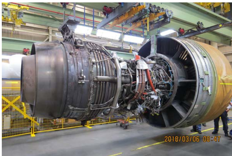
Photo No. 22: View of right side of engine showing no indications of an uncontainment, case rupture, or fire. (P&W)
