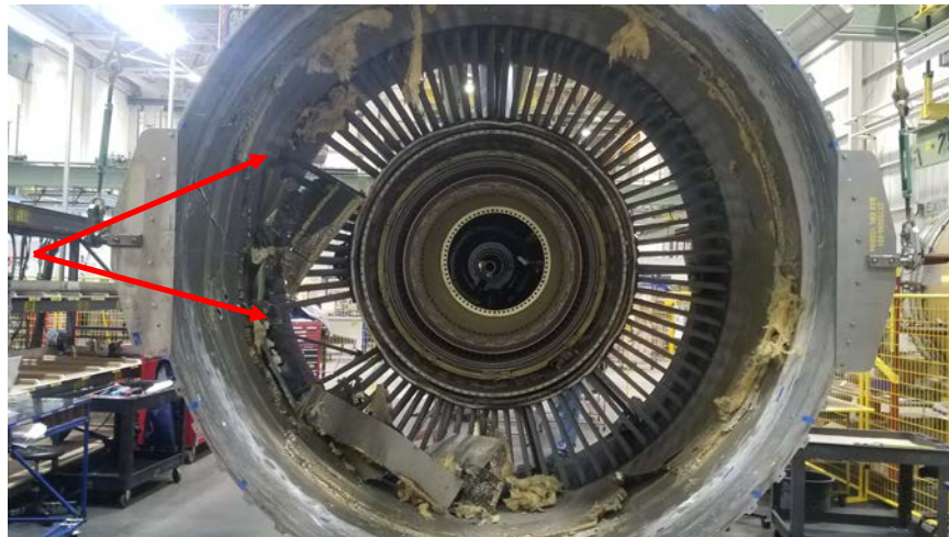
Photo No. 37: View of front of fan exit guide vanes showing locations of missing vanes. (Boeing)
