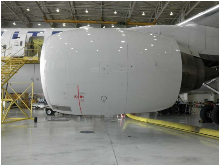
Photo No. 14: Left side of left engine showing exemplar inlet duct and cowling.
