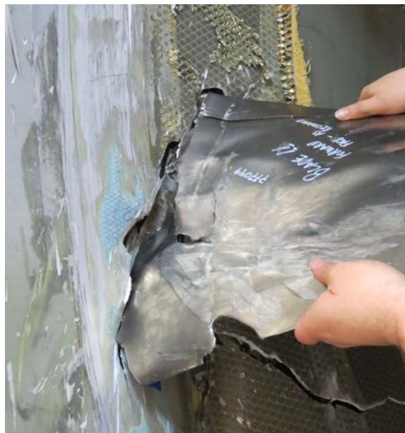
Photo No. 30: View of broken tip of fan blade No. 11 matched to hole in fan case. (P&W)
