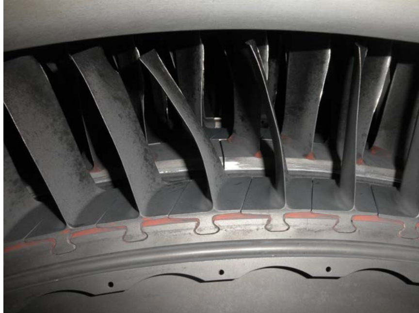
Photo No. 41: Close up of 4th stage LPC blades that were bent opposite the direction of rotation.
