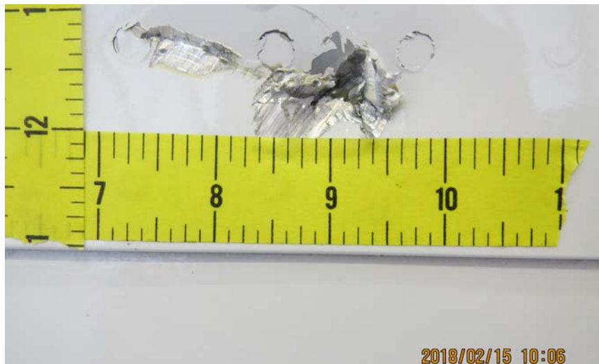
Photo No. 57: View of gouge in fuselage skin at BSTA 913. (P&W)
