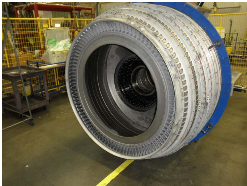
Photo No. 39: View of LPC drum showing that it is intact.
