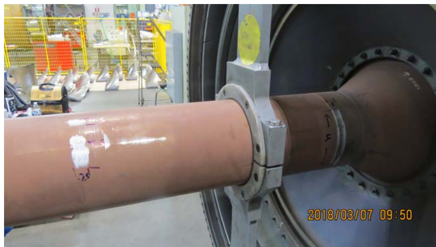
Photo No. 43: View of LPT shaft showing circumferential rub marks. (P&W)
