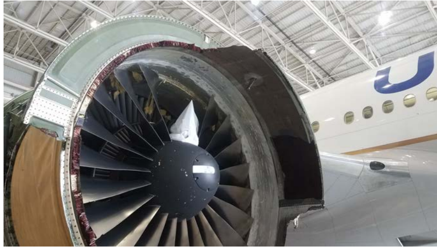
Photo No. 19: View showing that most of the upper inner barrel composite material remained attached to the aft bulkhead from about 9 to 12 o'clock. (Boeing)
