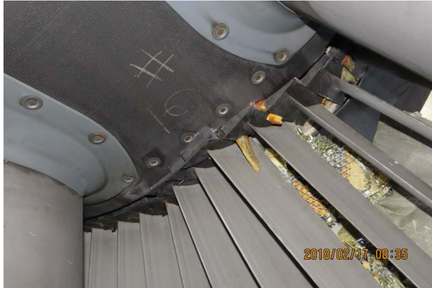
Photo No. 38: Close up view of inboard ends of fan exit guide vanes displaced rearward. (P&W)
