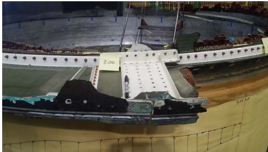
Photo No. 17: View of the aft bulkhead splice fitting showing no apparent damage. (Boeing)
