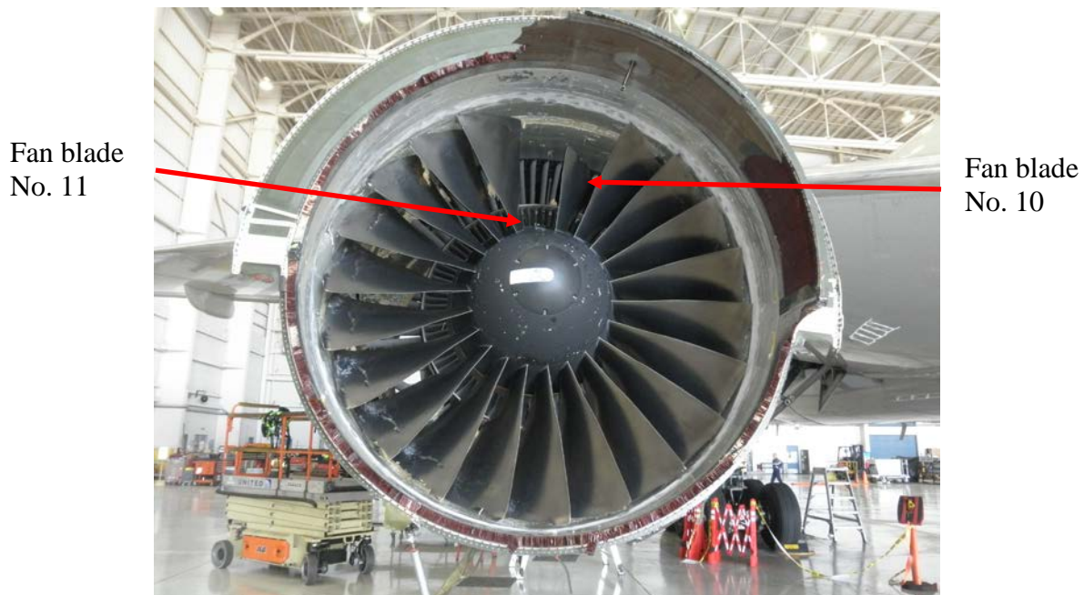
Photo No. 2: View of front of engine showing the two fractured fan blades, Nos. 10 and 11.
