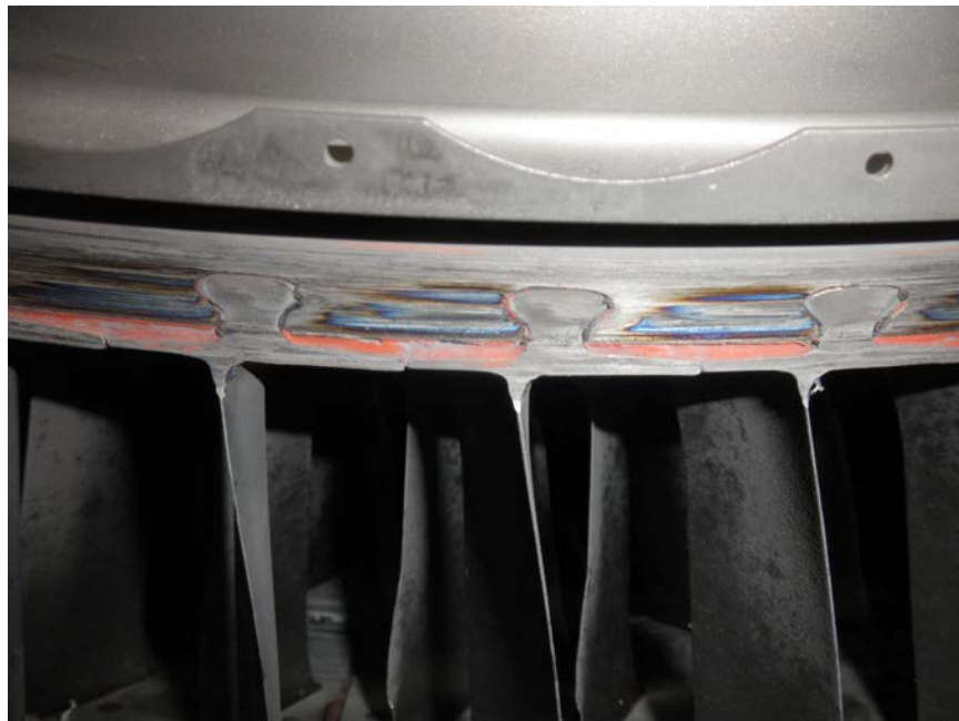
Photo No. 42: Close up of rub mark with heat discoloration on rear of LPC drum and 4th stage compressor blade roots.
