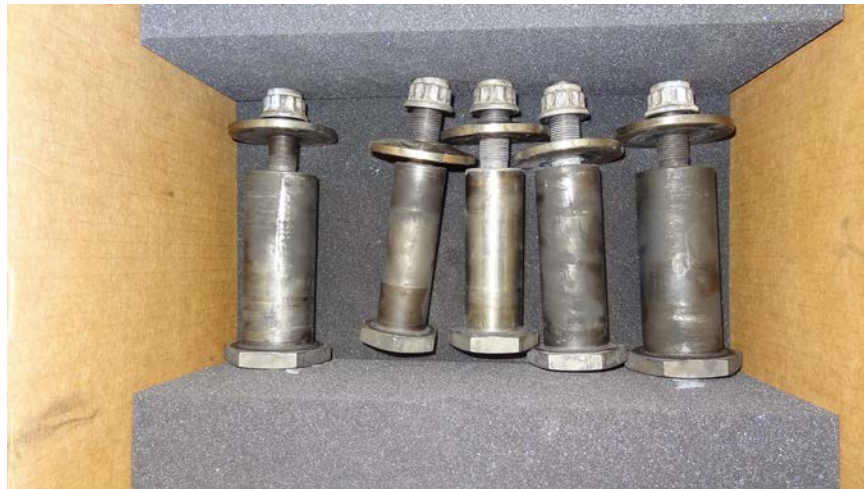
Photo No. 54: View of aft engine mount bolts. (Boeing)
