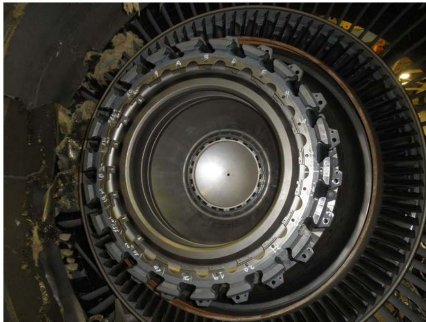
Photo No. 35: View of fan disk showing that it was intact.
