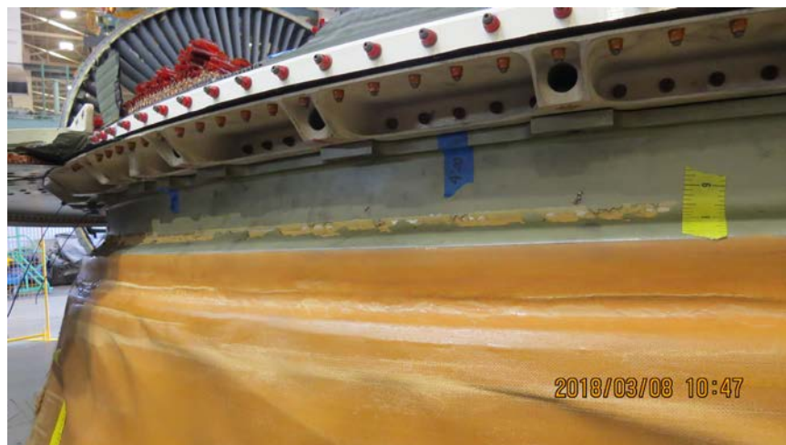
Photo No. 25: View of front of forward edge of Kevlar wrap showing chipped and cracked paint. (P&W)
