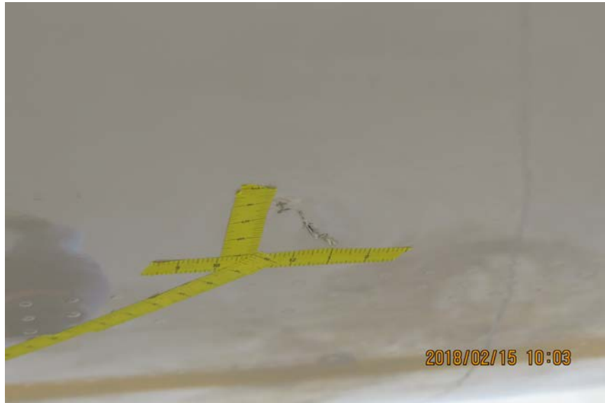
Photo No. 56: View of dent and crack in fuselage skin at BSTA 730. (P&W)
