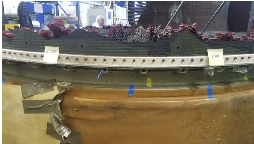
Photo No. 20: View of a portion of the lower inner barrel's composite panel that varied in length that remained attached to the aft bulkhead inner stiffener. (Boeing)
