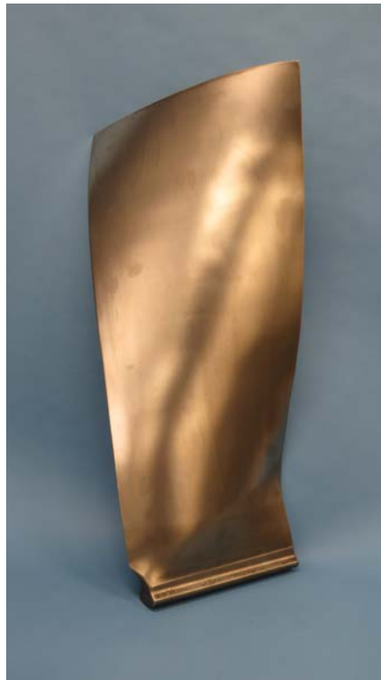
Photo No. 1: View of exemplar PW4000 112-inch fan blade. (P&W)
