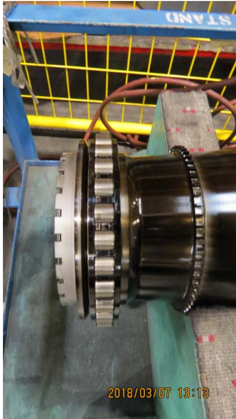
Photo No. 50: View of No. 1 1/2 bearing showing that it is wet with oil and did not have any rotational distress. (P&W)
