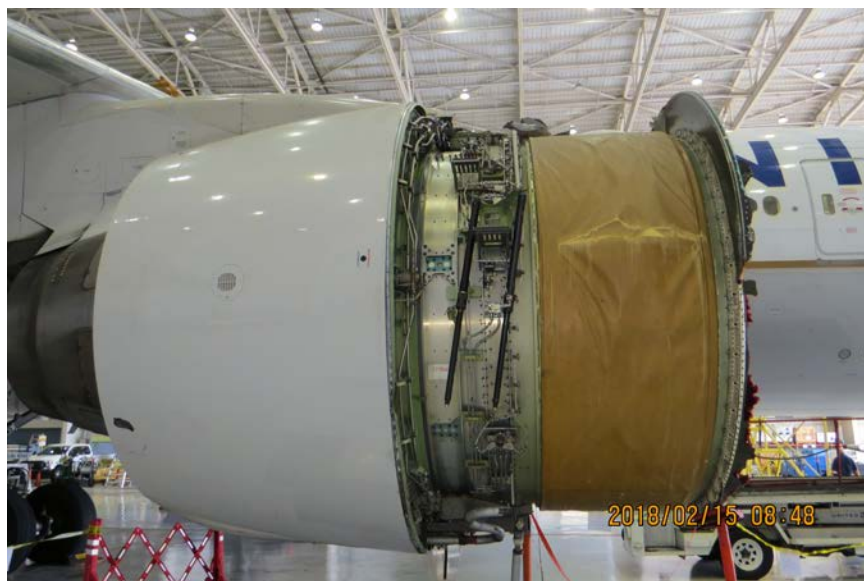
Photo No. 23: View of Kevlar wrap showing tear. (P&W)
