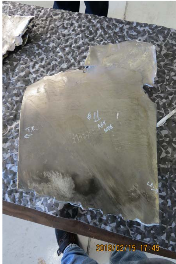
Photo No. 9: Fragment of fan blade No. 11 recovered from fan exit guide vanes. (P&W)
