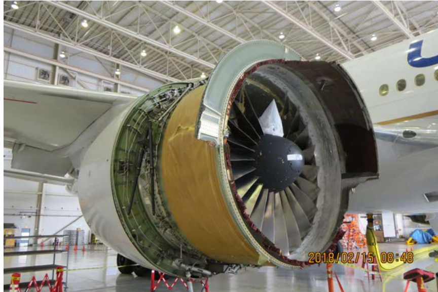
Photo No. 11: View of the right engine from the right front showing what remained of the inlet duct. White plastic was placed over the broken blades to protect the fracture surfaces. (P&W)
