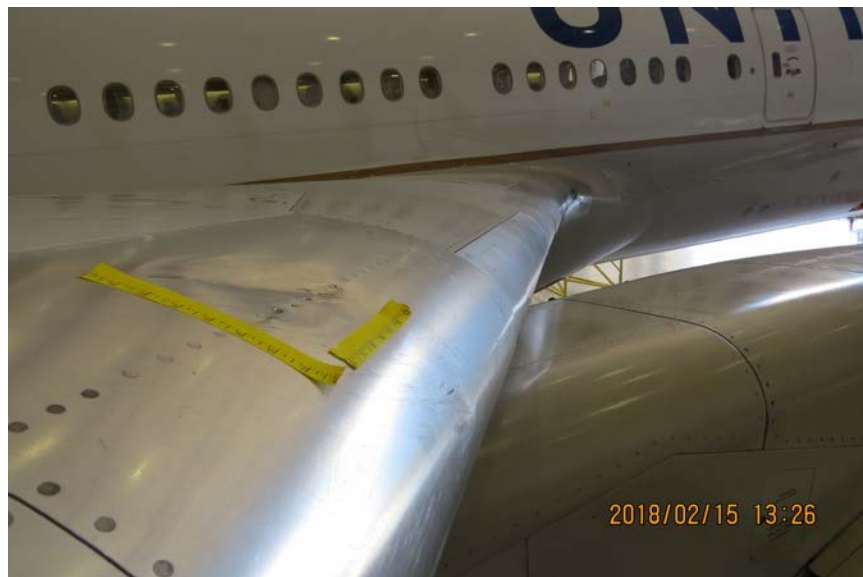
Photo No. 60: Dent in leading edge slat outboard of right engine. (P&W)
