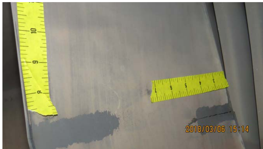
Photo No. 45: Close up of buckled turbine exhaust case strut showing leading and trailing edge cracks. (P&W)
