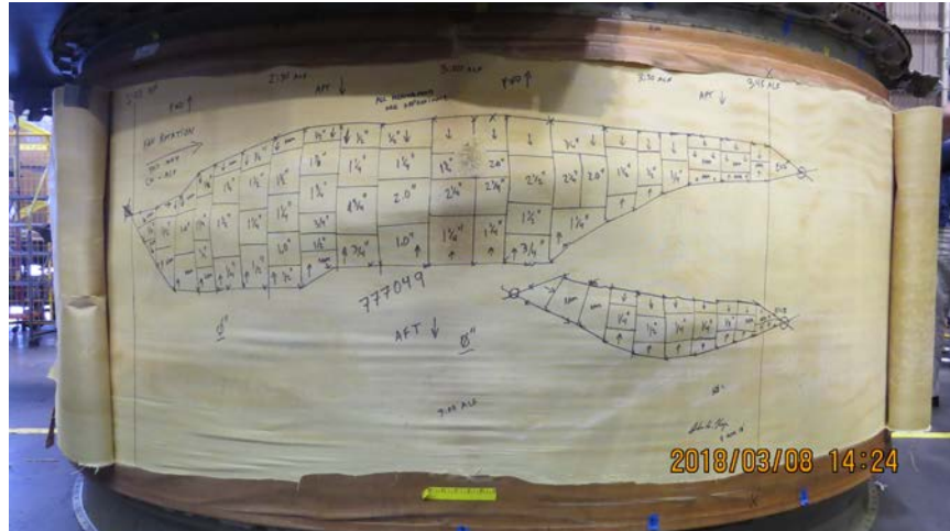
Photo No. 24: View of side of fan containment case showing deformation. (P&W)
