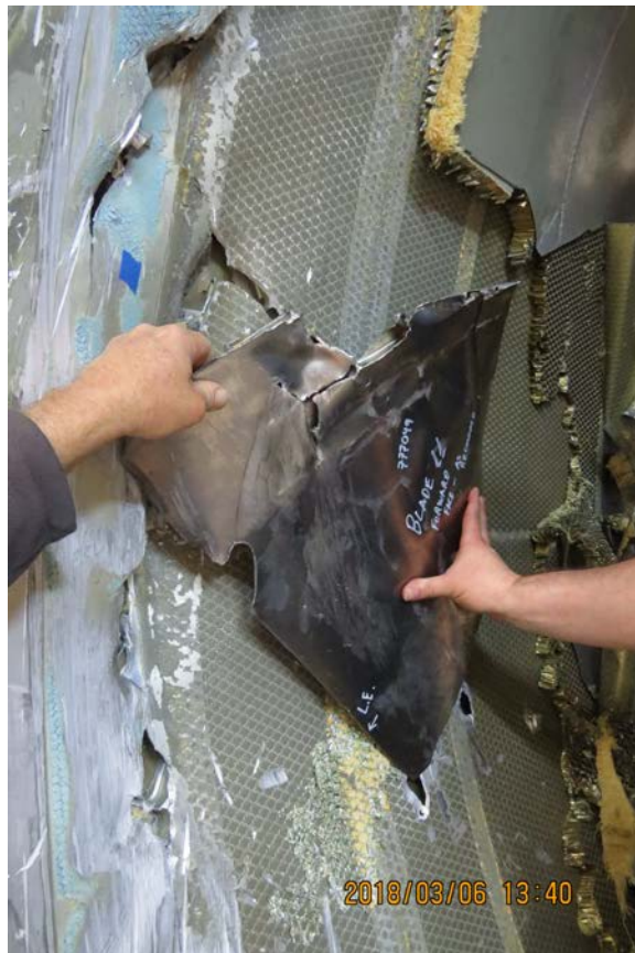
Photo No. 32: View of broken tip of fan blade No. 11 matched to second hole in fan case. (P&W)
