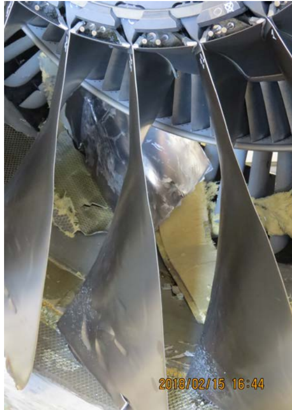
Photo No. 7: View between fan blades showing fragment of fan blade No. 11 against fan exit guide vanes. (P&W)
