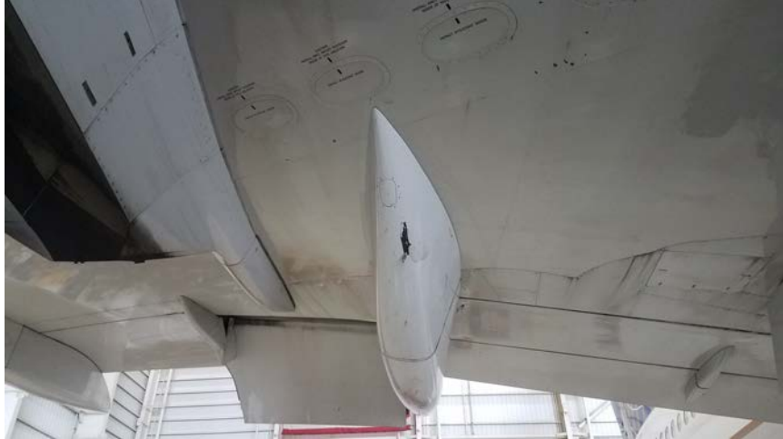
Photo No. 61: Gouge in the inboard flap's outboard flap track canoe fairing. (Boeing)
