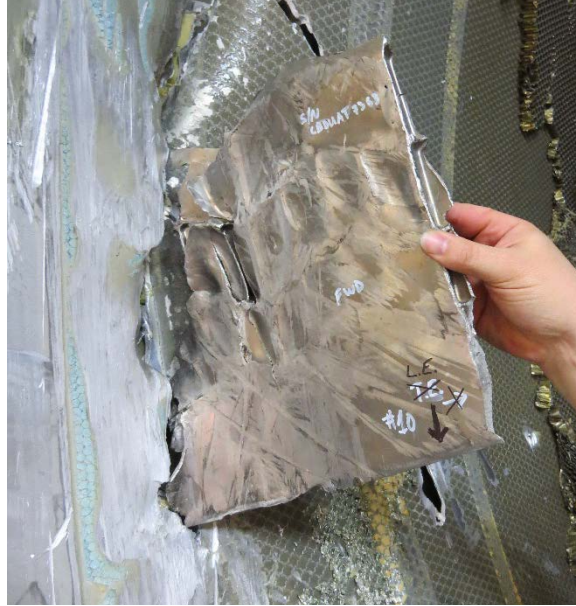
Photo No. 31: View of broken piece of fan blade No. 10 matched to hole in the fan case. (P&W)
