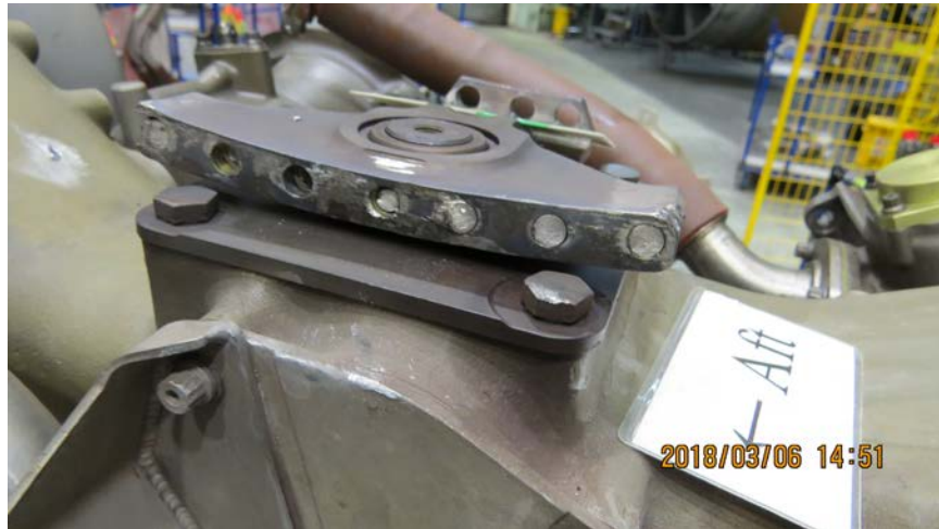
Photo No. 46: View of the engine gearbox attachment flange showing all seven mating bolts fractured. (P&W)
