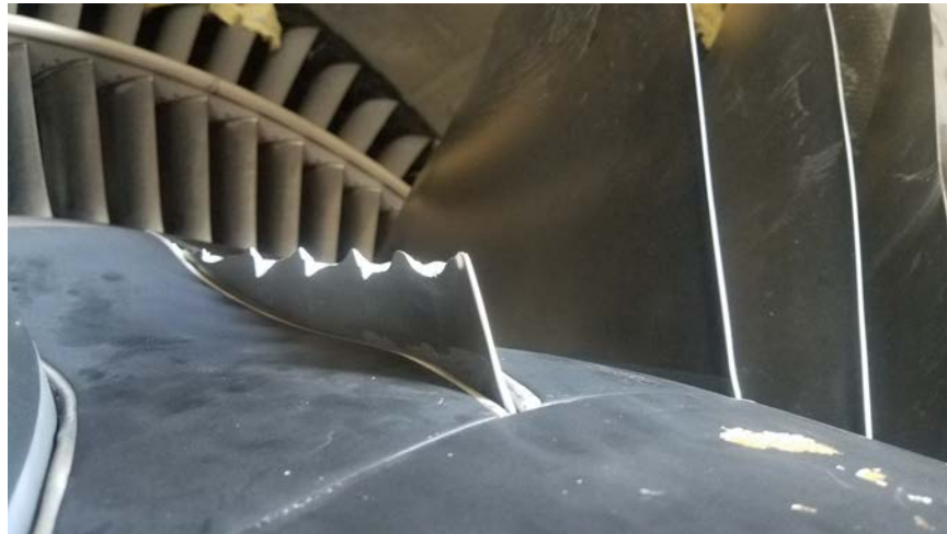
Photo No. 4: View of No. 11 fan blade showing sawtooth fracture pattern and the fracture surface being at about a 45° angle to the airfoil. (Boeing)
