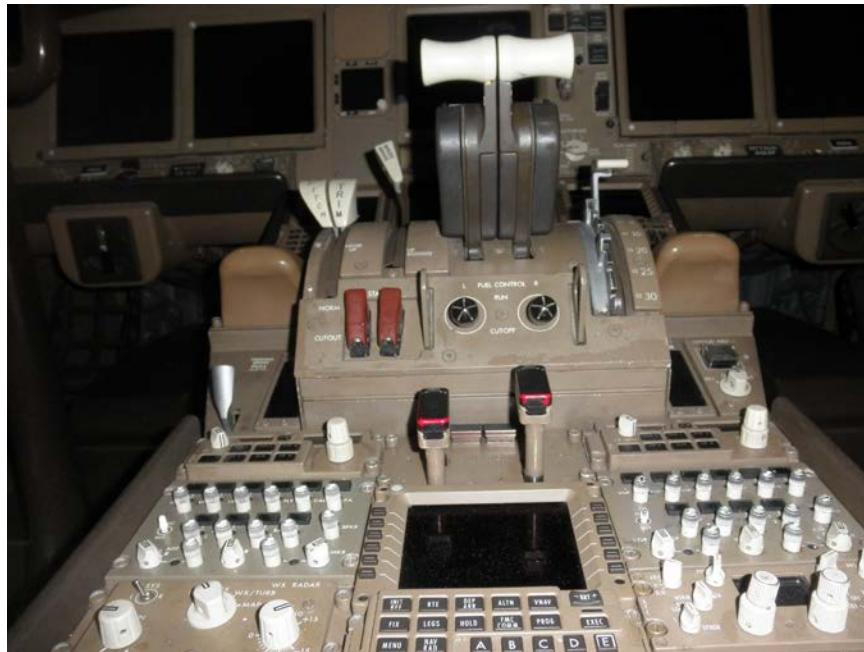
Photo No. 55: View of center console showing right engine's fire handle pulled up.
