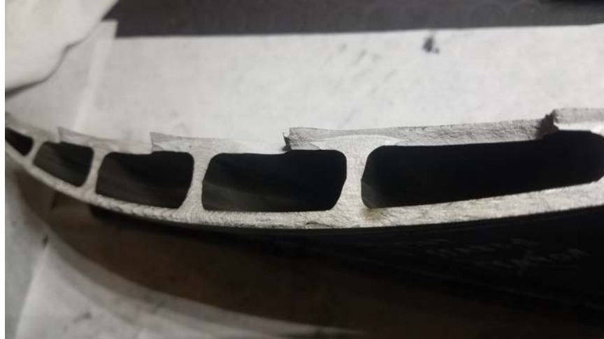
Photo No. 5: View of fracture surface showing elliptical marks and the internal ribs not being split. (Boeing)
