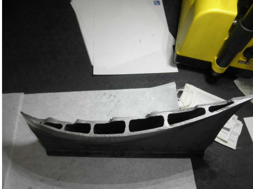
Photo No. 3: View of No. 11 fan blade showing fracture surface.
