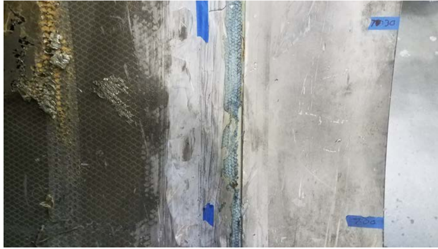
Photo No. 28: View of the fan blade rub strip showing the circumferential rub marks and the remains of the blue rub strip. (P&W)
