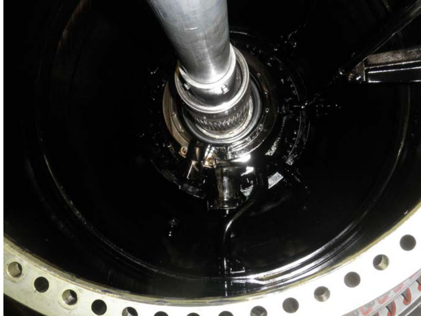
Photo No. 48: Interior of Nos. 1, 1 1/2, and 2 bearing compartment showing black color.
