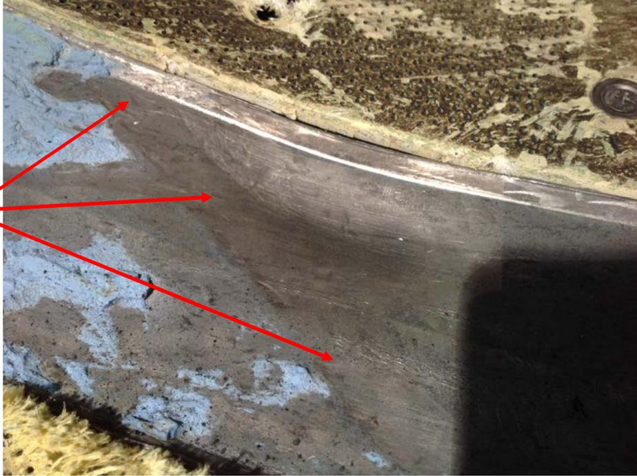
Photo 22 – Impact Through Abradable Material at 7:30 o'clock Location
