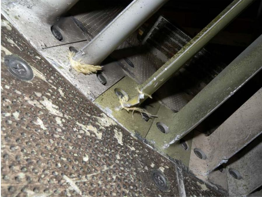
Photo 18 – OGV with embedded metallic debris
