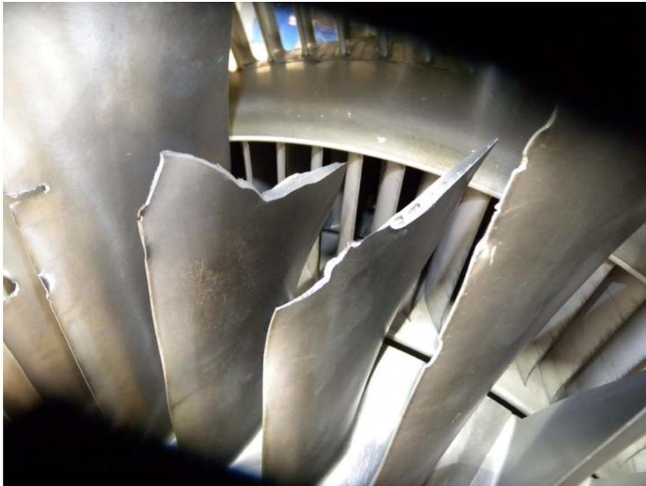
Photo 9 - Fractured Fan Blades – Close-up
