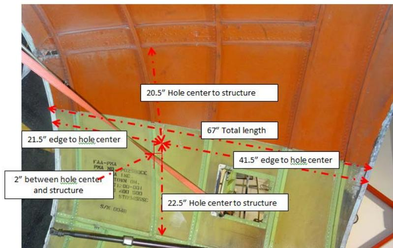
Figure 3 – Hole Locations in Outer Cowling
