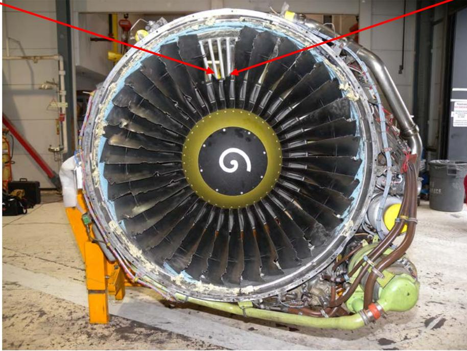
Photo 8 – Fractured Fan Blades – Close-up
