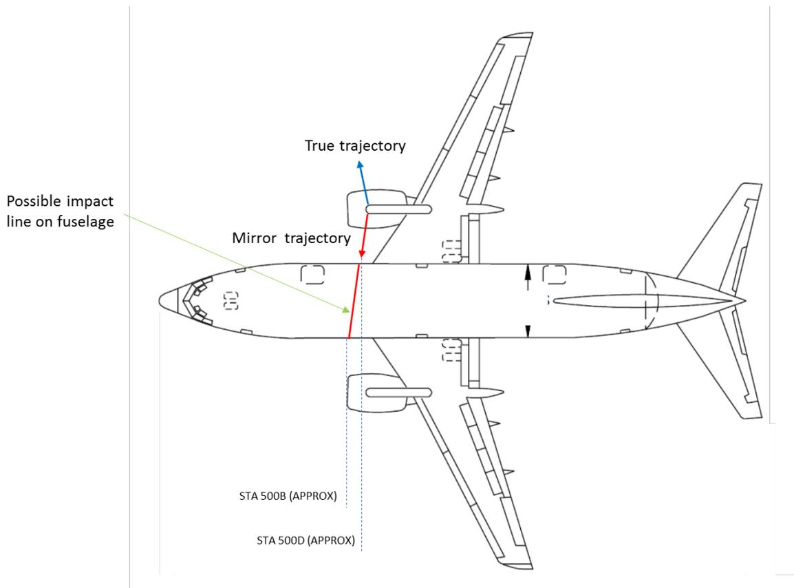
Figure 5 – Top View of Uncontained Fan Blade Particle Plane
