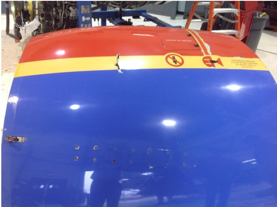
Photo 3 - 7-inch Long Penetration Tear - Detail
