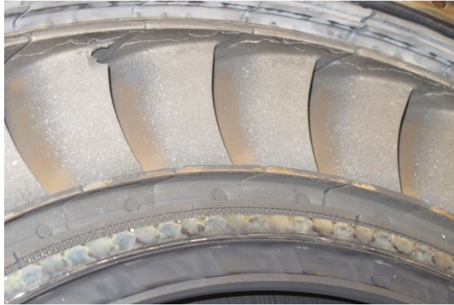
Photo 31- HPT 2 nd Stage Nozzle, Trailing Edge Impact Damage and Metal Spray
