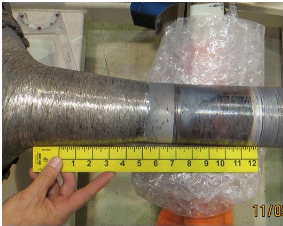
Photo 25- LPT Shaft- Gap Between Ruler and Shaft to Show Shaft Bend
