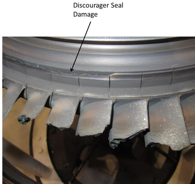
Photo 32- HPT 1 st Stage Blade Tip Damage
