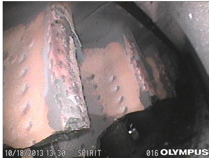
Photo 17- HPT 1 st Stage Blade Airfoil Tip Damage
