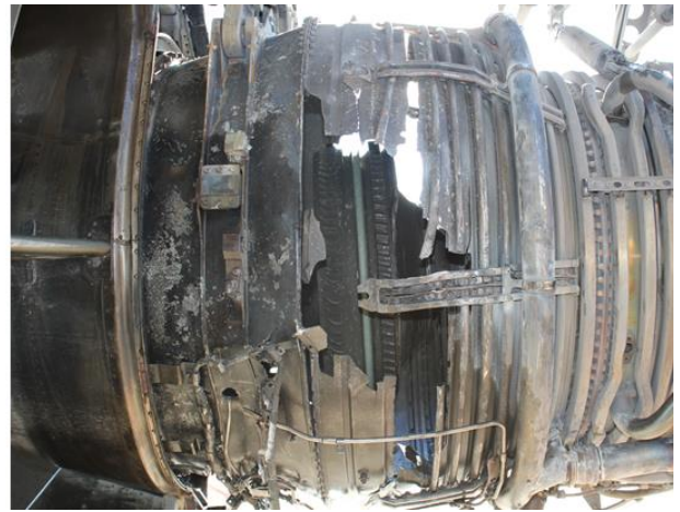
Photo 6- LPT and TEC Damage (L) Left Side of Engine (R) Right Side of Engine
