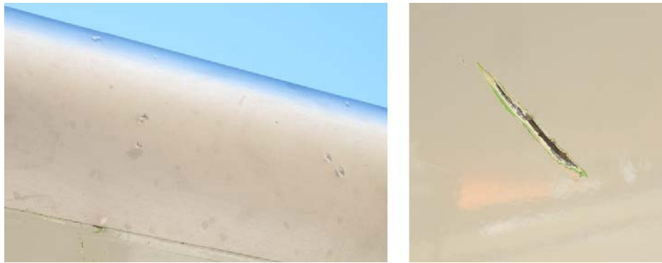
Photo 3- Impact Marks on the Horizontal Stabilizer Leading Edge
