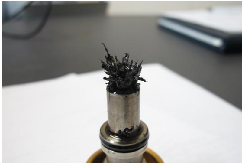
Photo 2- Main Chip Detector Plug with Metal Shavings and Debris
