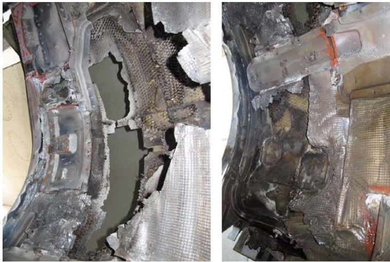
Photo 11- Missing Material and Thermal Damage to Left Side C-Duct
