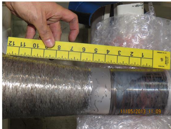
Photo 25- LPT Shaft- Gap Between Ruler and Shaft to Show Shaft Bend
