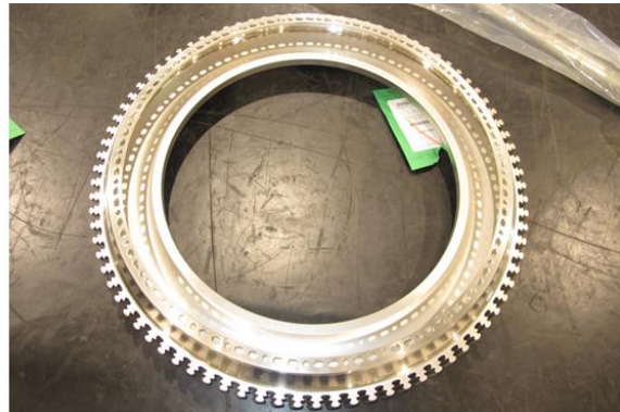
Photo 26- LPT 5 th Stage Disk, (L) As Removed From Engine (R) New Disk
