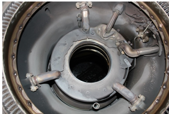
Photo 35- No. 4 Bearing Forward Compartment Heat Shield Damage
