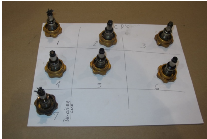
Photo 20- Magnetic Chip Detector Plugs, Main Oil Tank (1) and De-Oiler Plugs (7) With Debris
