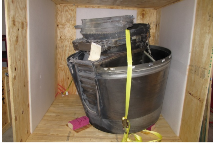
Photo 19- Turbine Exhaust Case and Common Nozzle Assembly- As Received
