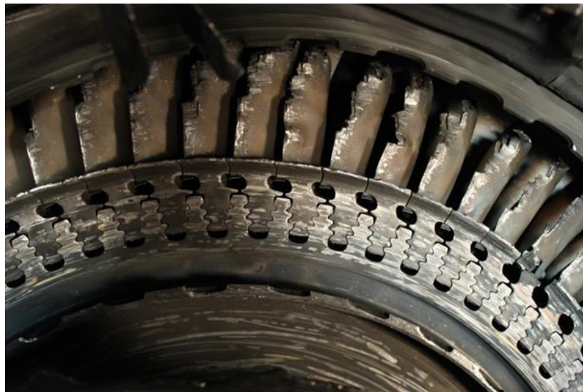
Photo 13- HPT 2 nd Stage Turbine Disk Damage
