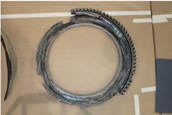
Photo 26- LPT 5 th Stage Disk, (L) As Removed From Engine (R) New Disk
