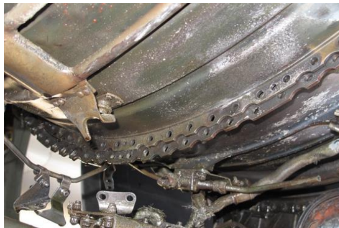
Photo 10- P Flange Shift Between LPT Case and Turbine Exhaust Case
