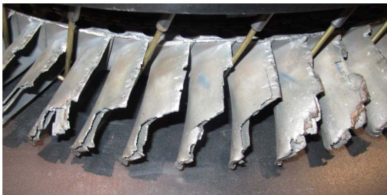
Photo 30- HPT 2 nd Stage Blade Damage, Blades Secured in Fixture
