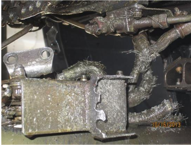
Photo 8- EGT Harness Junction Box, Damaged Harness
