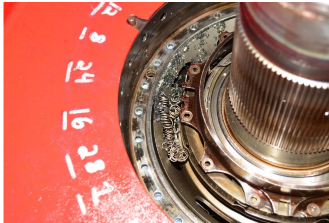
Photo 34- No. 4 Bearing Aft Compartment Debris
