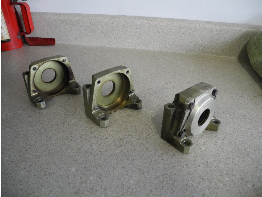
Photo 7 – Engine Mounts – Two Fractured and Without Elastomer
