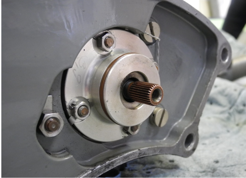
Photo 17 - FCU Input Drive Splined Drive - Undamaged
