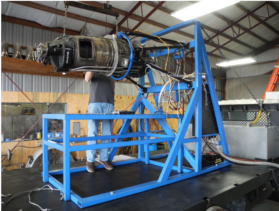
Photo 8 – TPT Truck Frame Mounted Test Cell
