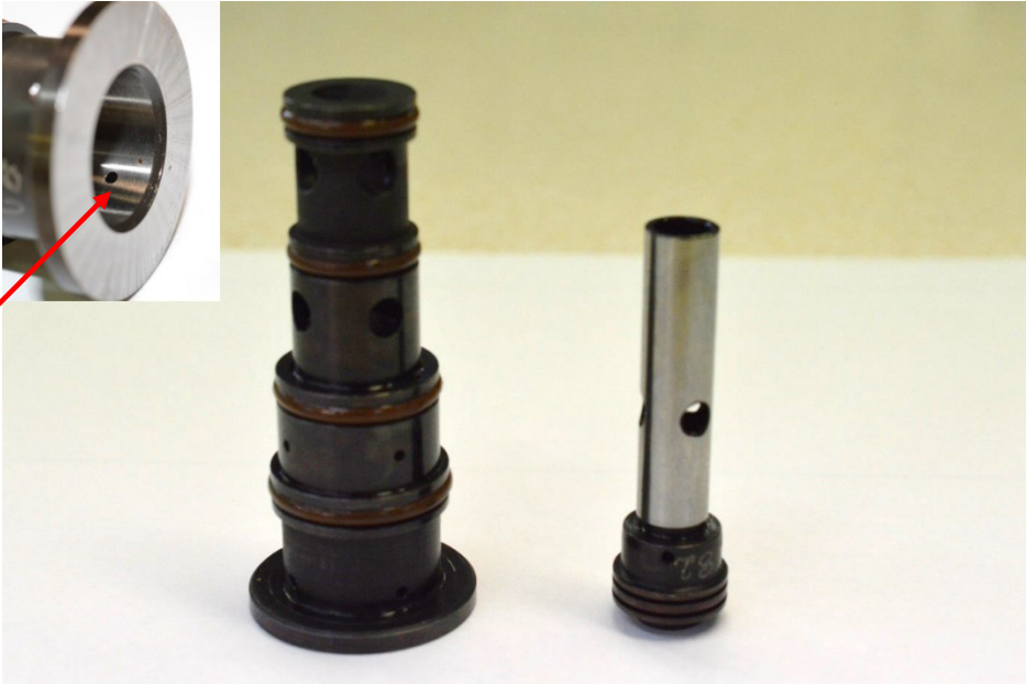
Photo 28 - Fuel Cutoff Valve
