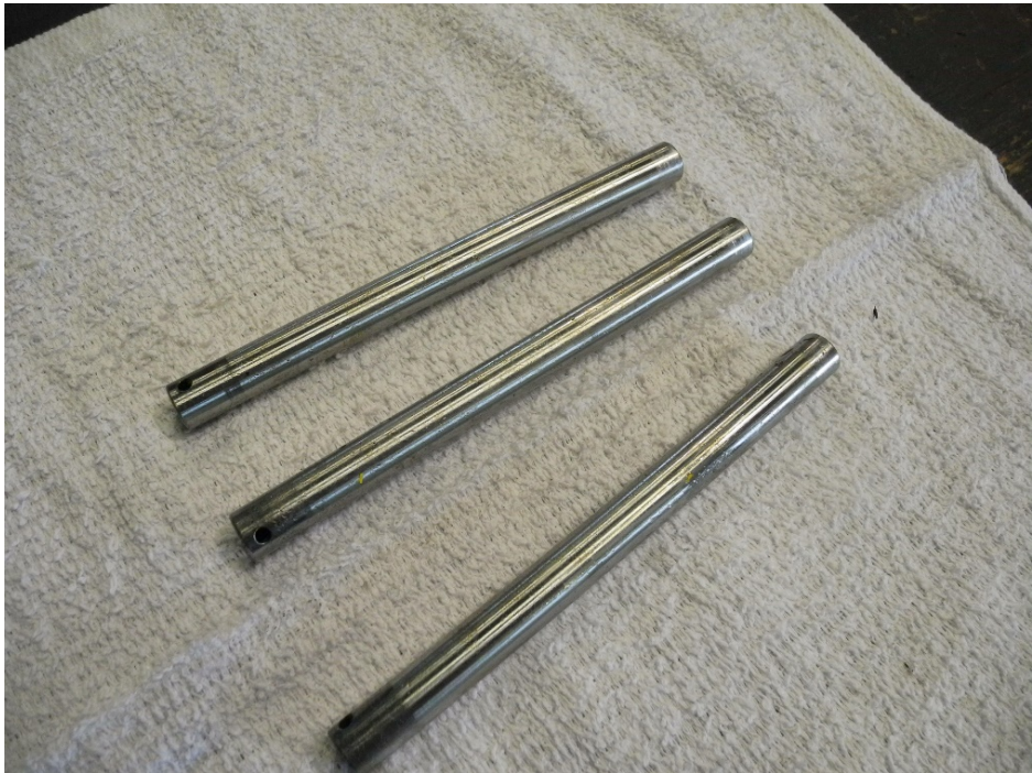
Photo 65 - Fork Guides - Undamaged
