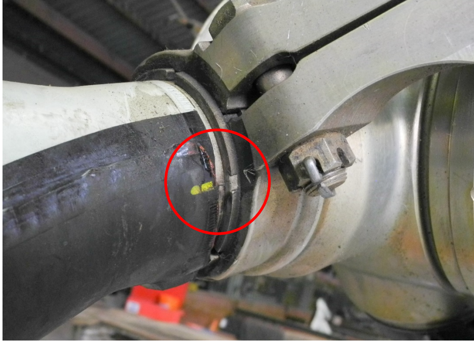
Photo 51 - Blade #3 – Alignment Scribe Marks - Aligned
