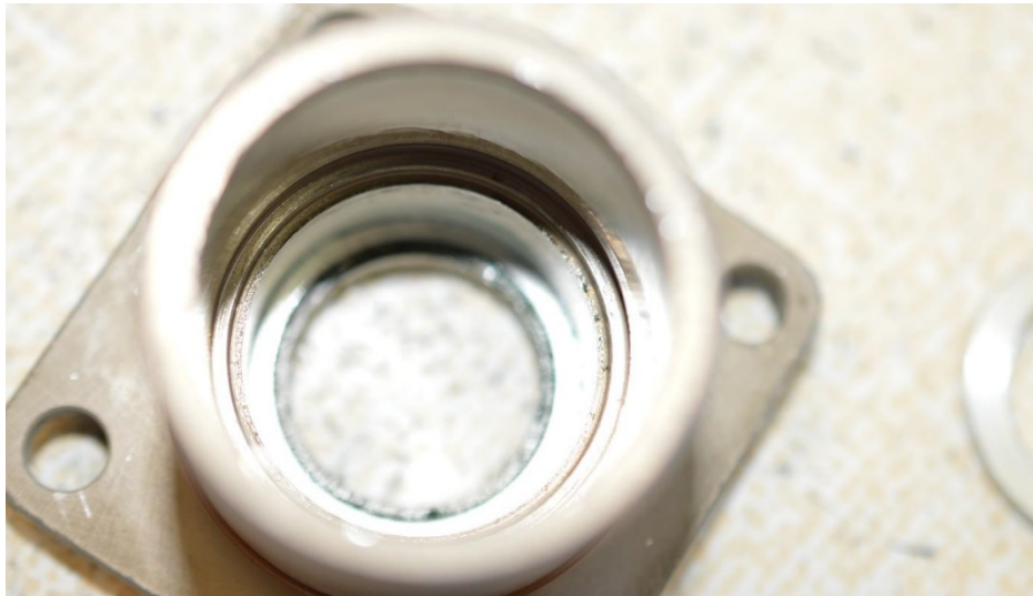
Photo 22 – Alpha Shaft Housing – Reworked Retain to Non-Standard Seal
