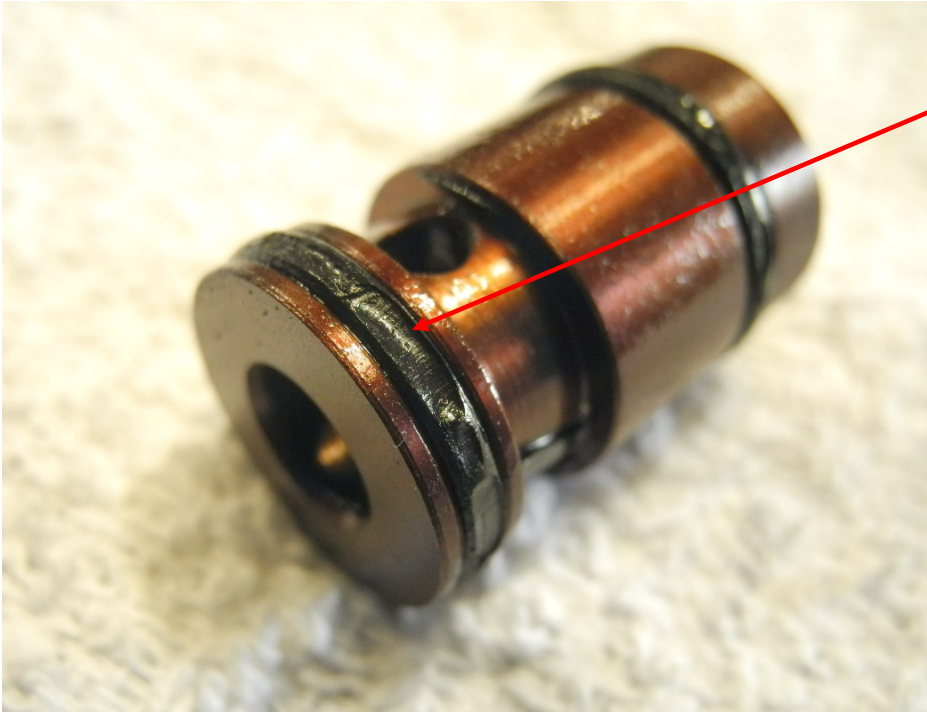
Photo 64 - Aft Spacer of the Pitch Lock Components
