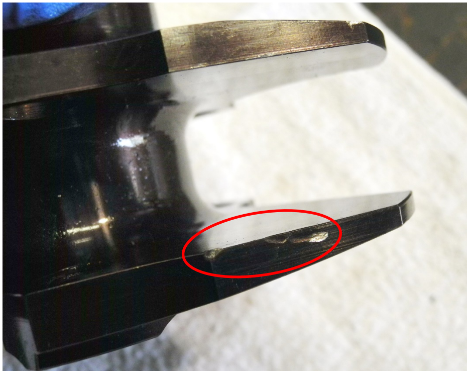
Photo 68 - Fork Front Surface - Dented
