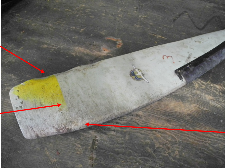
Photo 47 – Typical Damage to Blades
