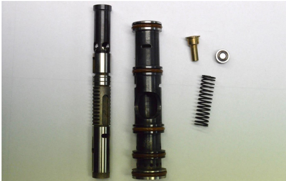
Photo 26 - Emergency Metering Valve Assembly
