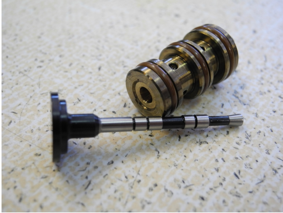
Photo 25 - Main Fuel Valve – Intact & Undamaged
