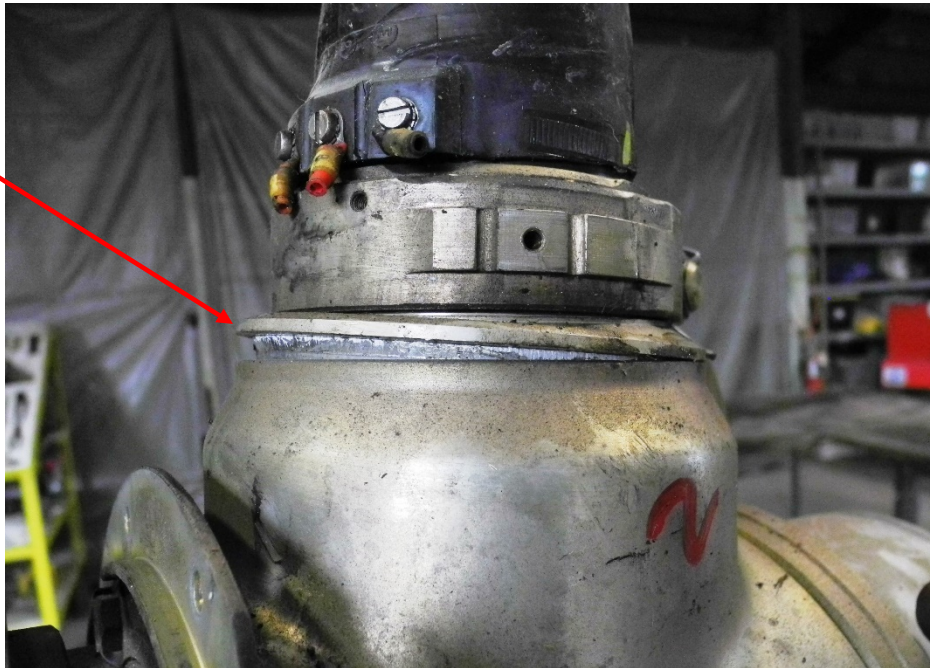
Photo 52 - Bearing Ring Blade #2 – Flange is Sheared
