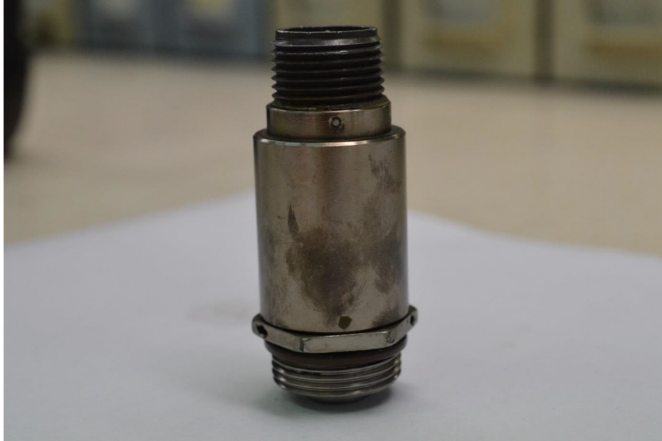
Photo 29 - Emergency Circuit Solenoid
