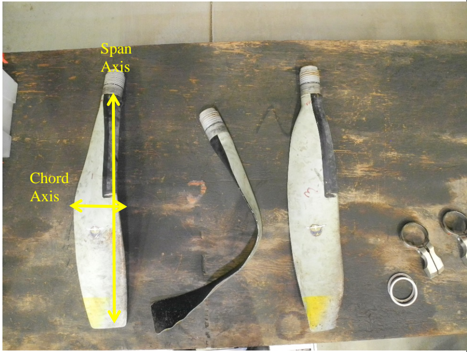
Photo 46 - Propeller Blades – General Damage
