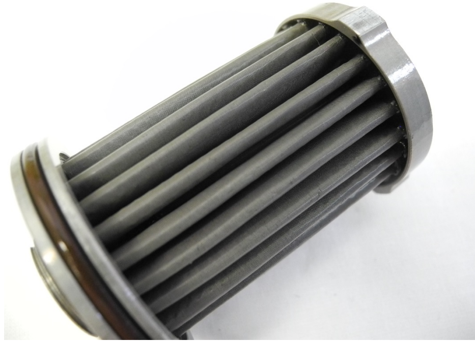
Photo 33 - Fuel Filter Element - Clean
