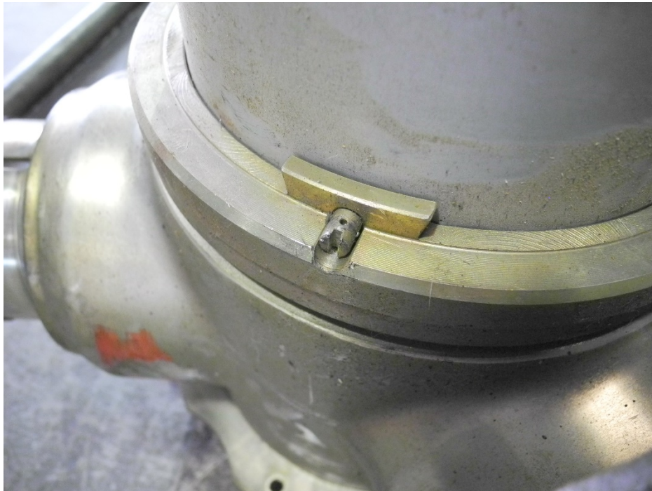
Photo 58 - Cylinder Lock Screw – Lockwire Removed
