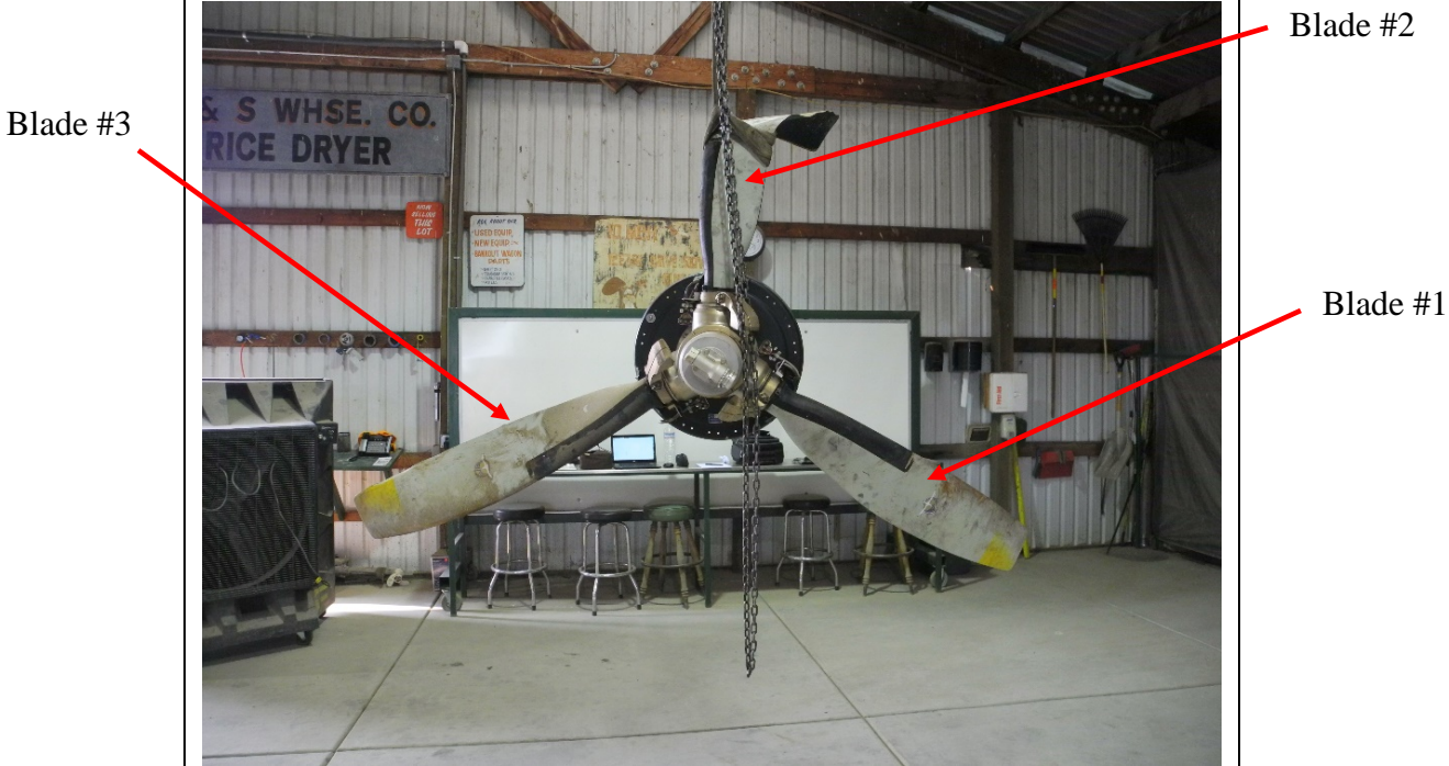
Photo 45 – AVIA Propeller - V508E/84/B2, S/N 140651237
