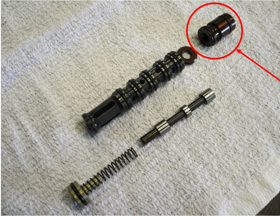
Photo 63 - Secondary Pitch Lock Components - Intact
