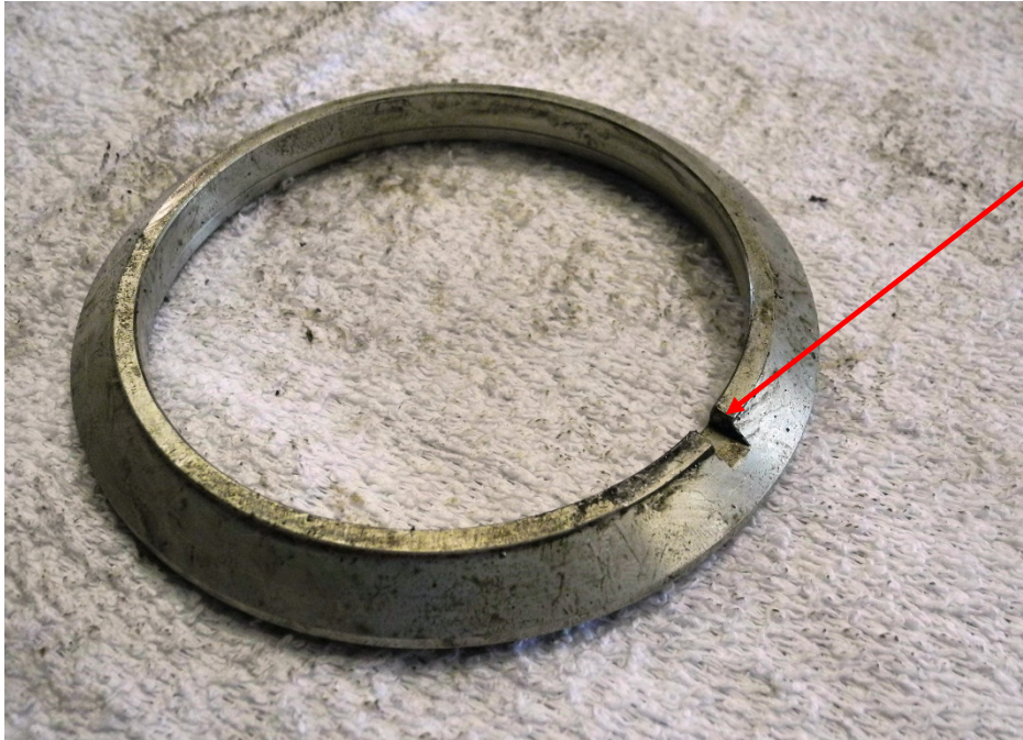
Photo 53 - Bearing Ring of Blade #3 - Undamaged
