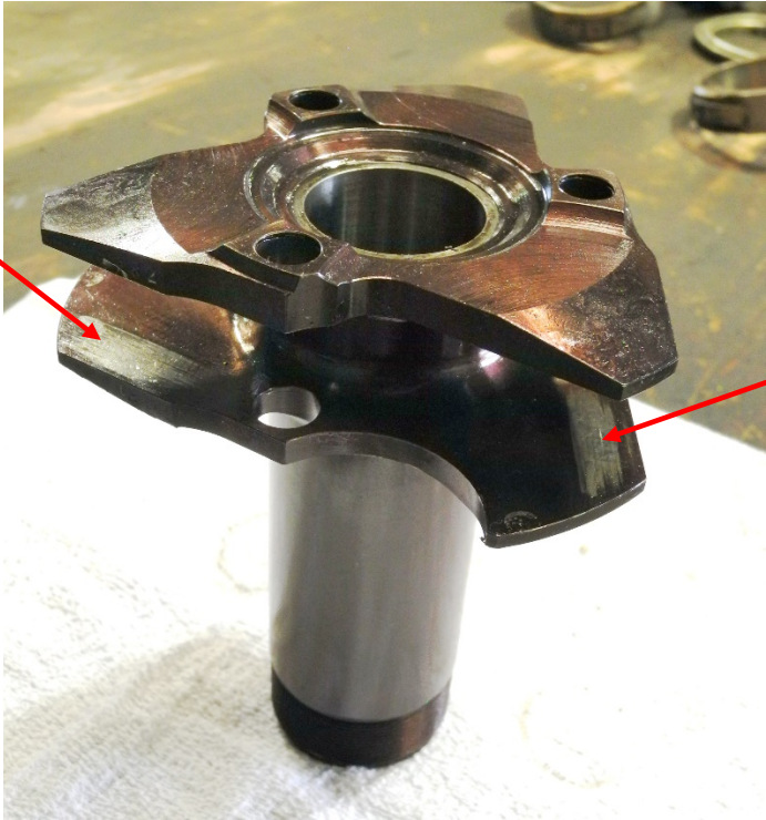
Photo 66 - Fork – Wear from Pitch Change Blocks
