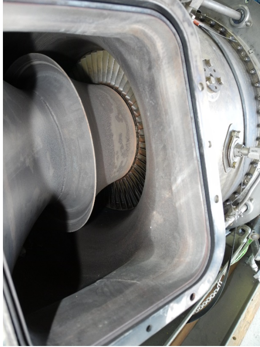
Photo 3 – Power Turbine Blades - Undamaged
