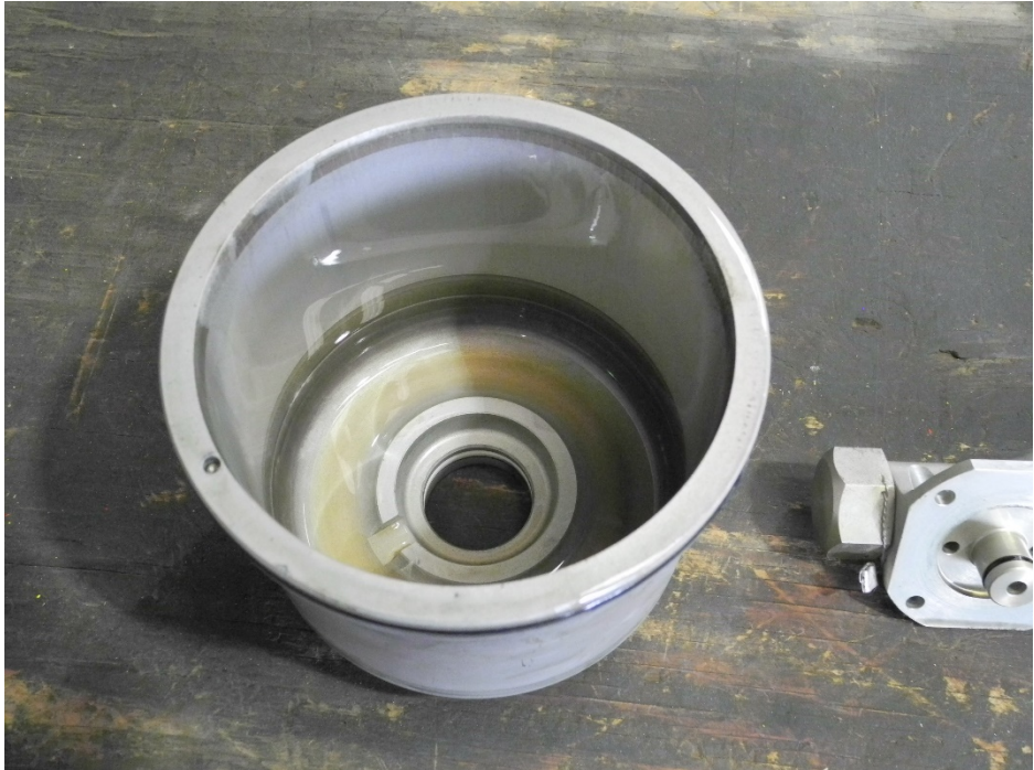
Photo 59 - Inner Surface of Cylinder - Undamaged
