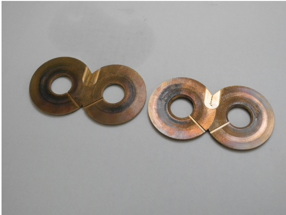
Photo 38 - Brass Side Sealing Plates - Undamaged
