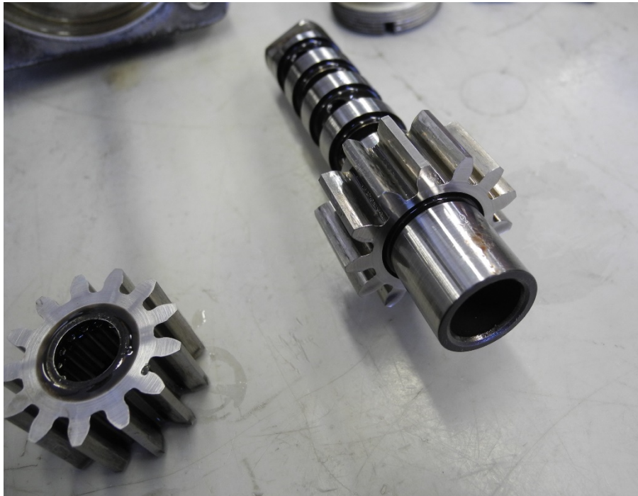
Photo 42 - Oil Pump Involute Gear Teeth - Undamaged
