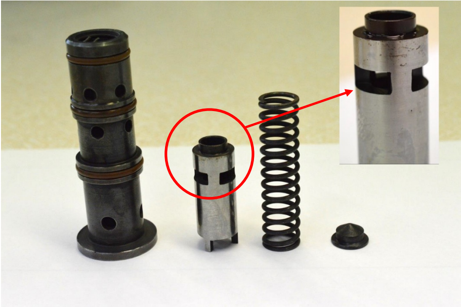
Photo 27 - Pressure Regulating Valve of the Emergency Circuit – Minor Corrosion
