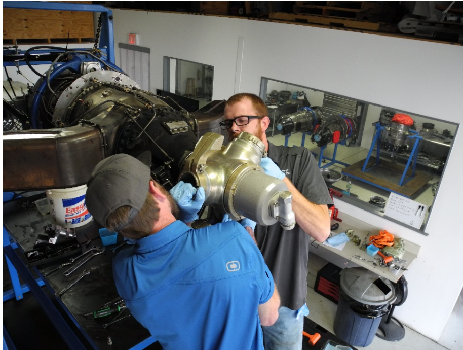
Photo 10 – Mounting Slave Propeller
