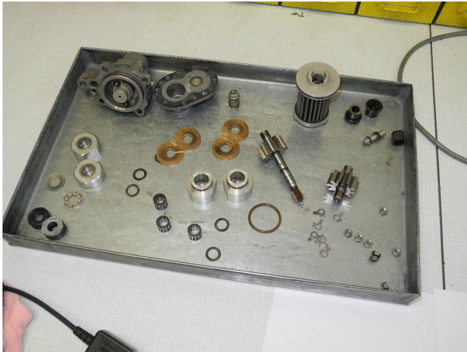
Photo 36 - Fuel Pump - Disassembled
