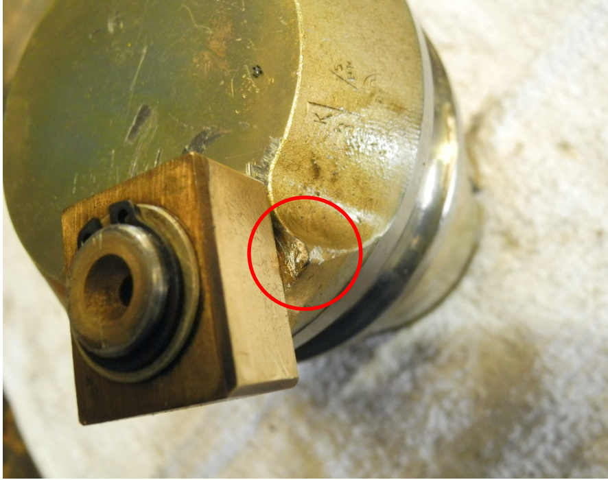
Photo 71 - Blade Bushing – Impact Marks
