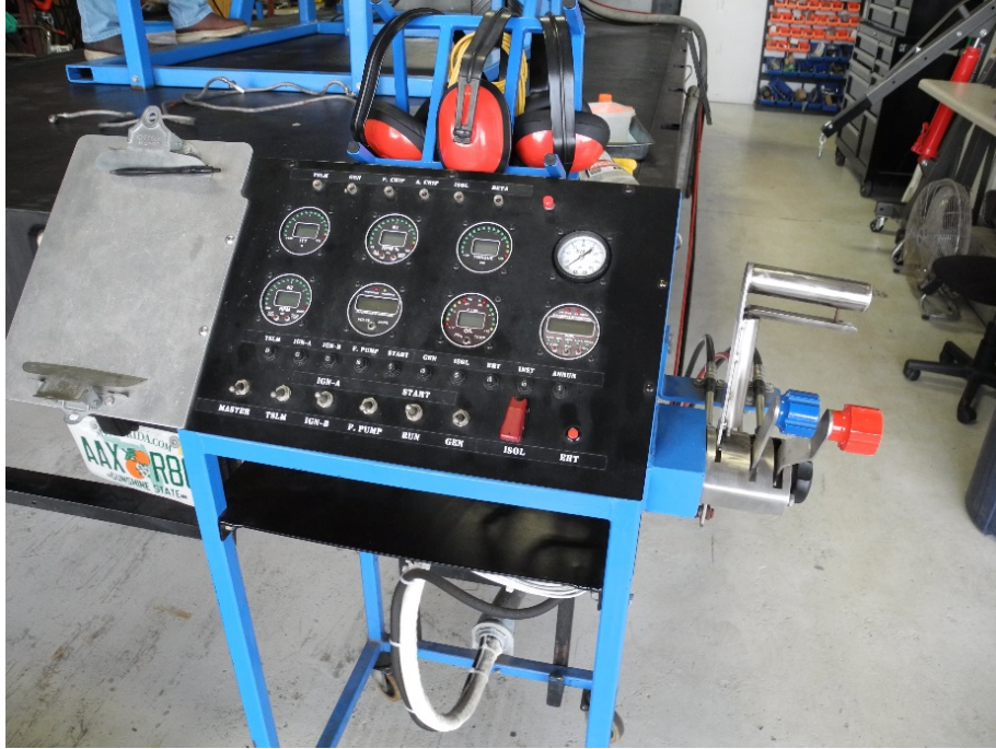
Photo 9 – TPT Truck Frame Mounted Test Cell – Control Panel
