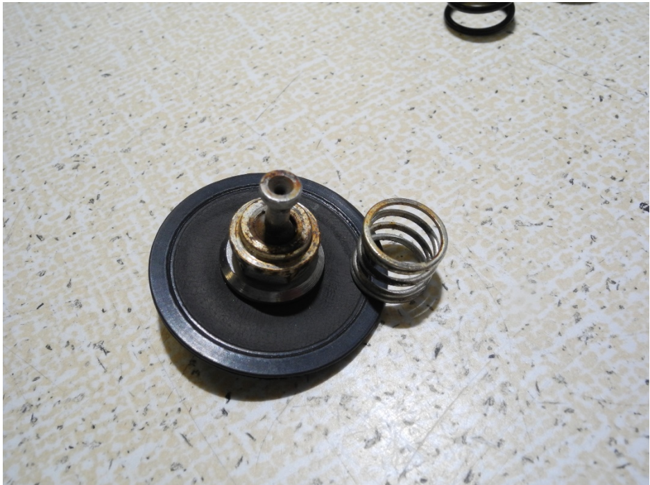
Photo 23 - Rubber Diaphragm and Spring - Corroded
