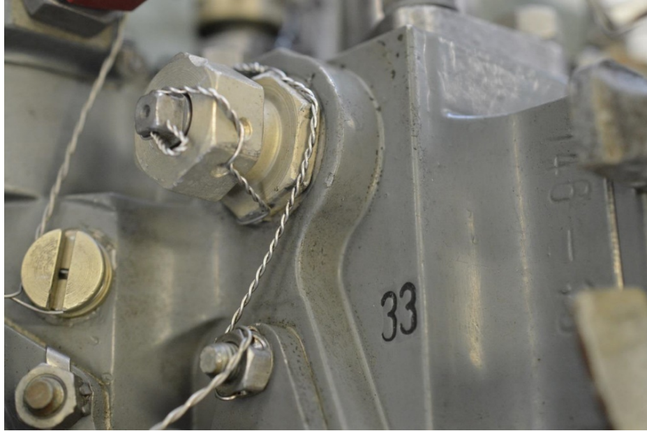
Photo 19 - Lock Wire at adjustment Screw 33
