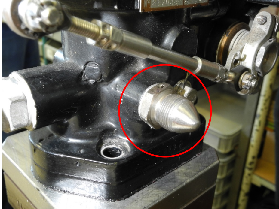
Photo 41 - Emergency Feather Fitting Blanked-off
