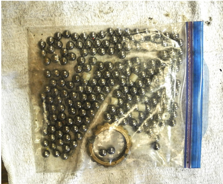
Photo 70 - Blade Bushing Ball Bearings - Undamaged
