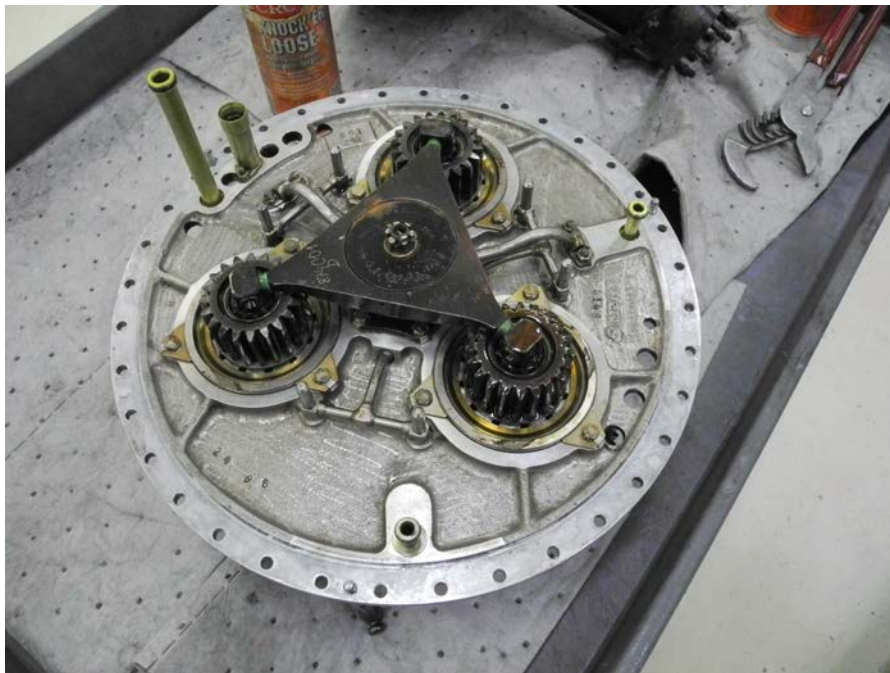
Figure 24 – Reduction Gear Support Diaphragm
