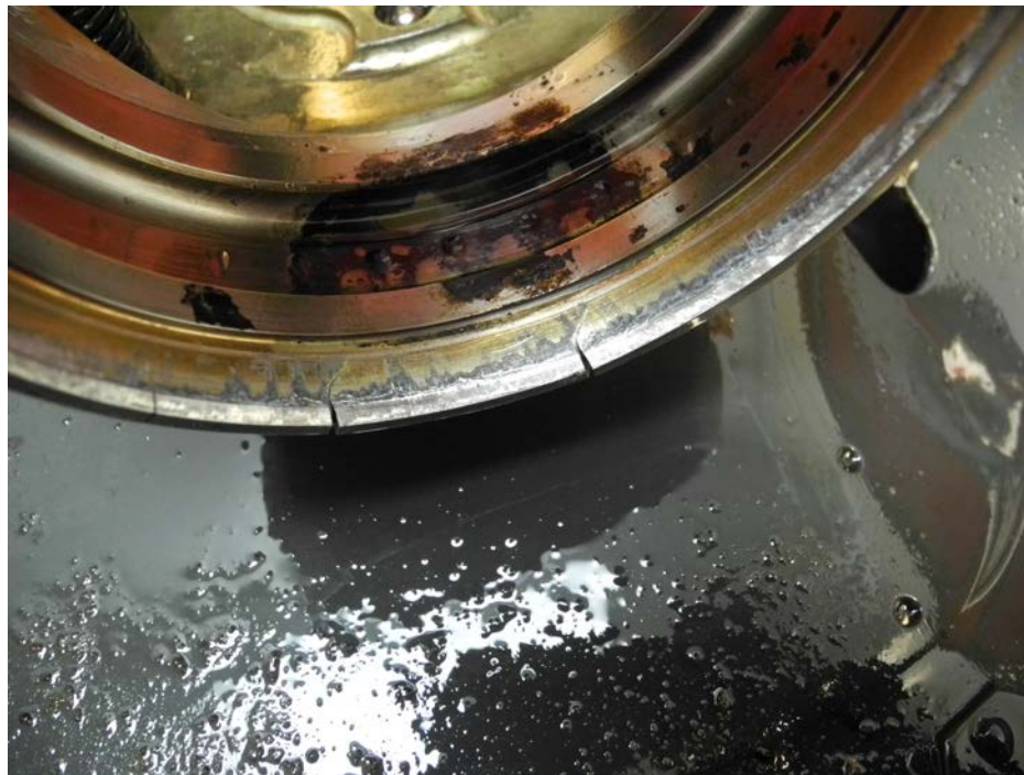
Figure 74 – Blade Bushing Sleeve – Fractured
