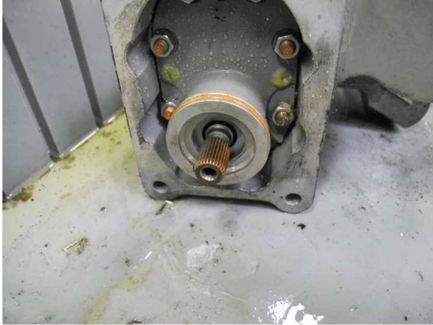
Figure 45 - Fuel Pump Input Drive Spline - Undamaged
