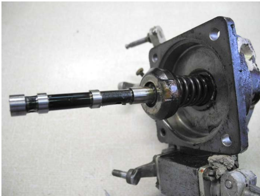
Figure 60 – Pilot Valve & Speeder Spring - Undamaged
