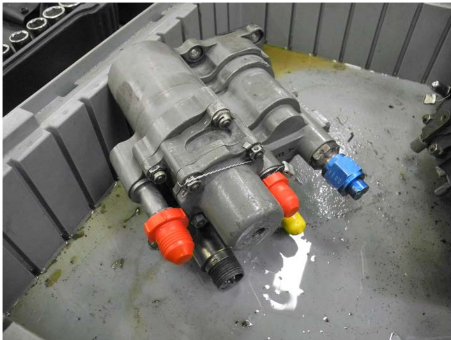
Figure 44 - Fuel Pump - Jihostroj, P/N LUN6290.03.8, S/N 873 026
