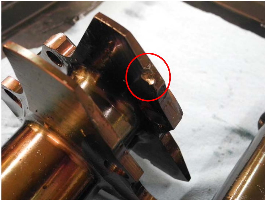
Figure 71 – Impact Dent from Contact Against Pitch Change Block
