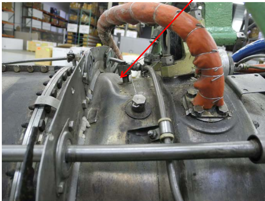
Figure 9 – Gas Generator (GG) Case - Buckled
