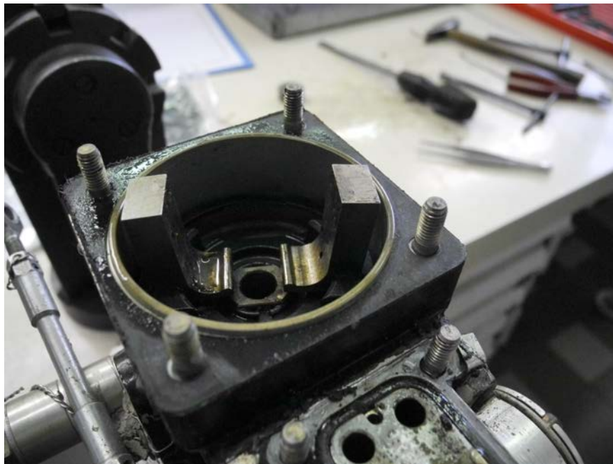
Figure 61 – PCU Flyweights – Undamaged and Free to Operate
