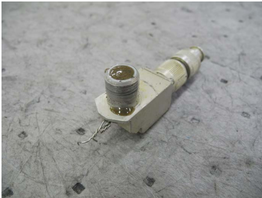
Figure 14 – RGB Chip Detector – Water Contaminated
