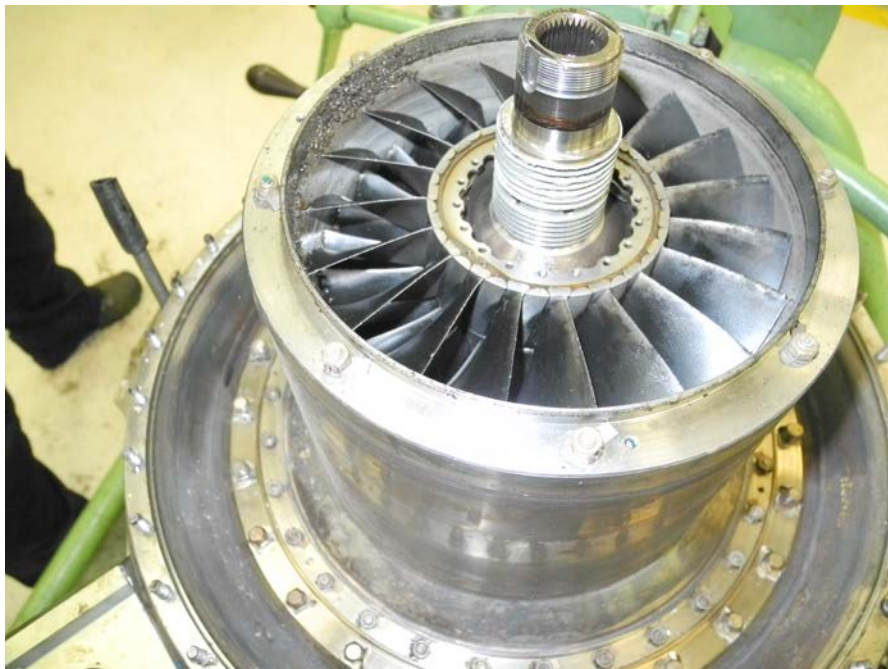
Figure 36 – 1 st Stage Compressor Rotor
