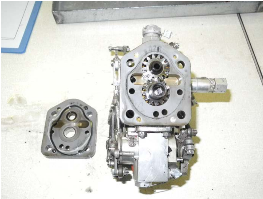
Figure 59 – PCU Involute Gears and Side Seals - Undamaged
