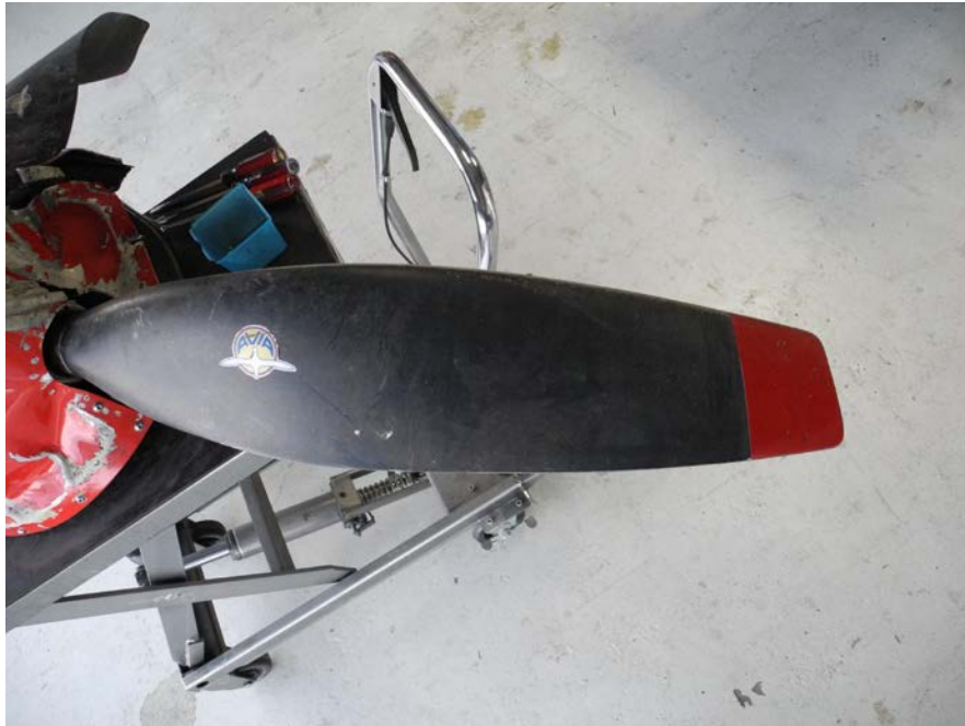
Figure 64 – Blade – No Impact or Scoring Damage
