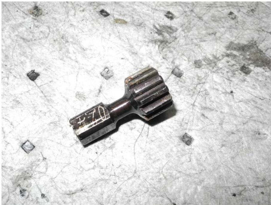
Figure 58 – Propeller Control Unit Input Drive Spline - Undamaged
