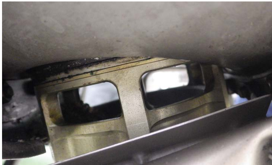
Figure 12 – Compressor Air Bleed Valve (ABV) - Open
