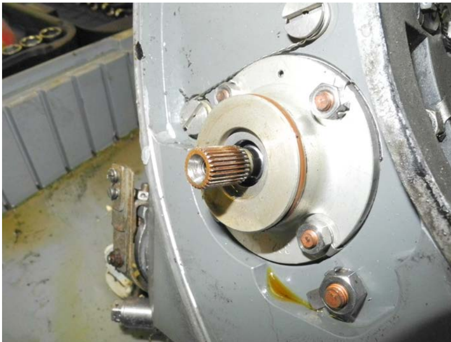
Figure 50 – Fuel Control Unit Input Drive Spline - Undamaged
