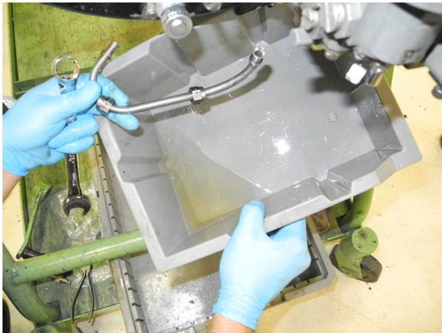
Figure 22 – Fuel Collected from FCU and Associated Tubing
