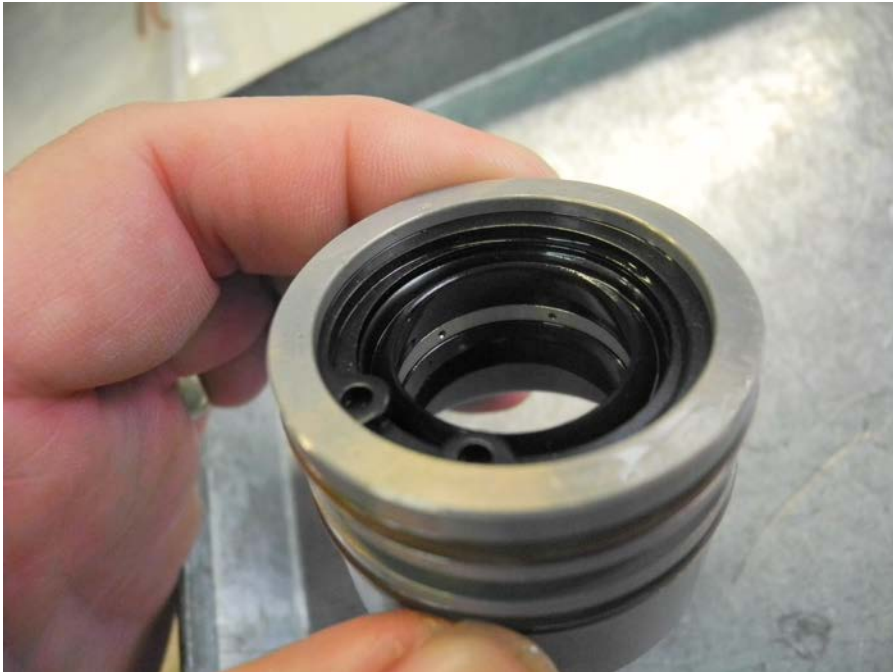
Figure 54 - Main Metering Valve Bearing Sleeve Seal - Undamaged
