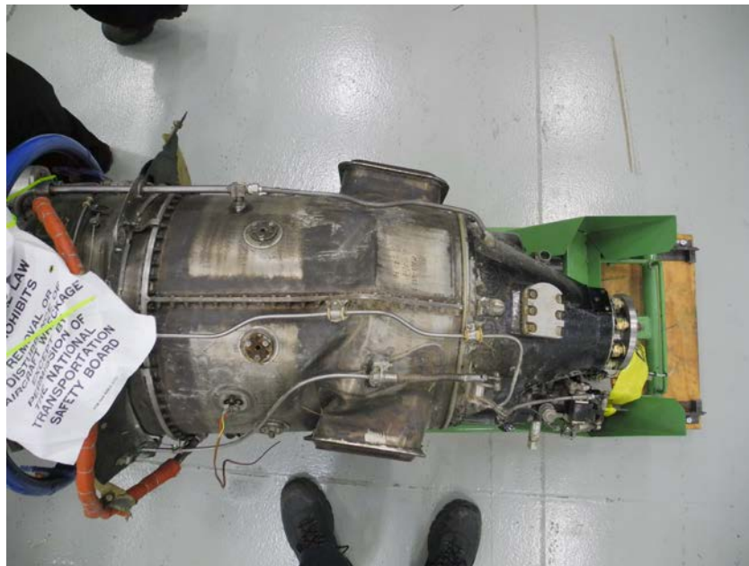
Figure 8 – Exhaust Case Deformation
