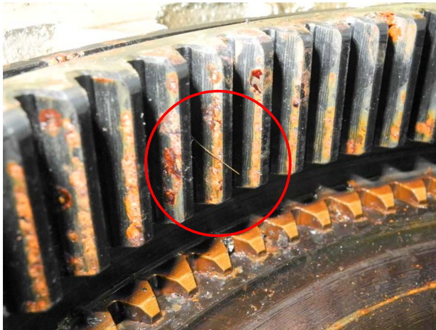
Figure 28 – Magnetic Sliver in Ring Gear Teeth
