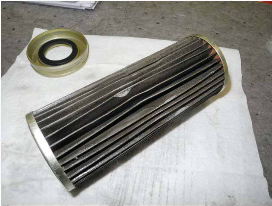
Figure 17 – Oil Filter – Free of Metallic Particles
