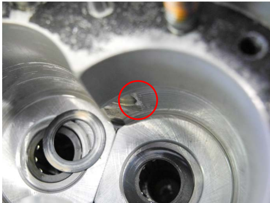
Figure 48 - Cavitation On Pump Gear Housing Inlet Edges
