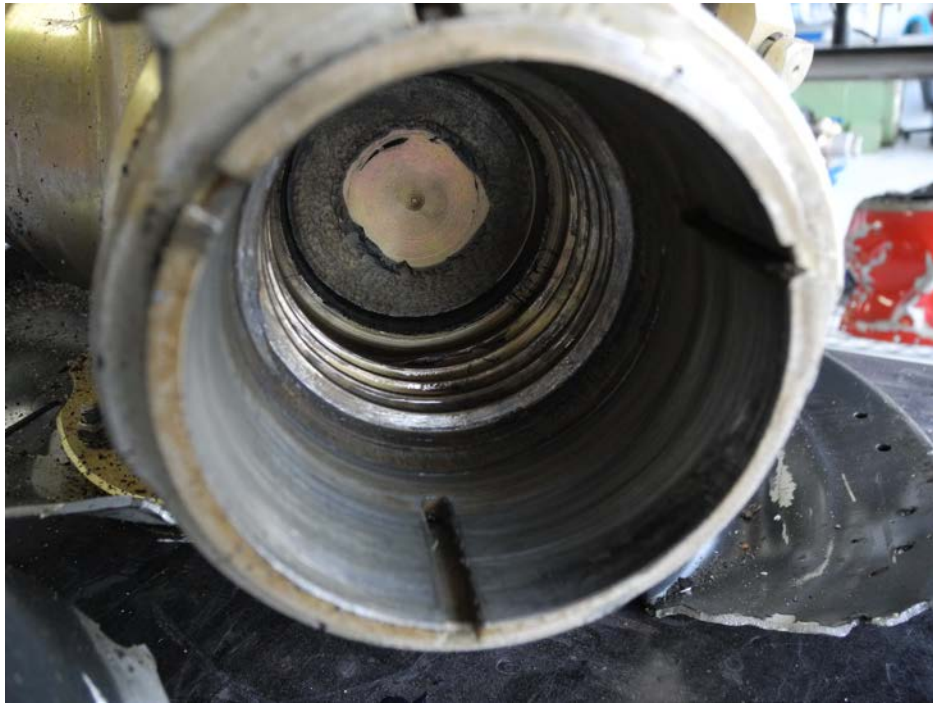
Figure 67 – Blade Bushing - Undamaged
