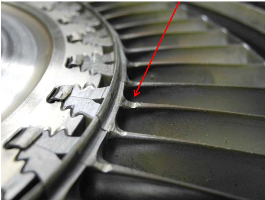
Figure 30 - Power Turbine - Rotationally Scored Near Blade Root
