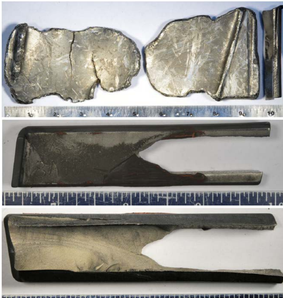
Photo 9- Fractured No. 1 Fan Blade Recovered in Three Pieces
