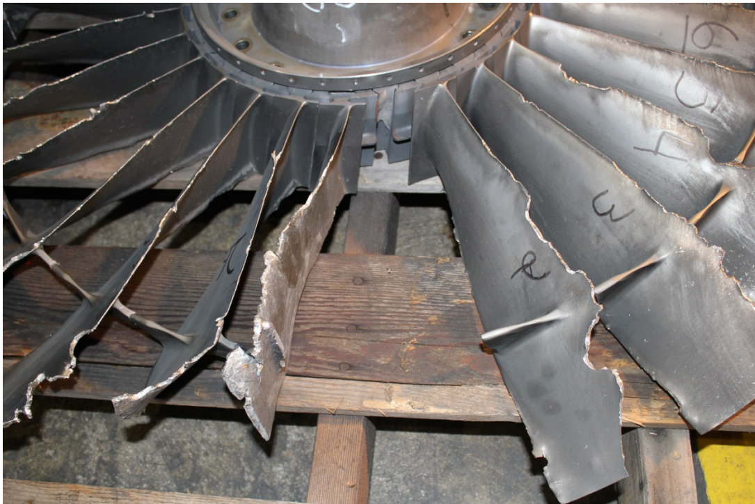
Photo 8- Fractured Fan Blade, Blade Root Still Present in Slot
