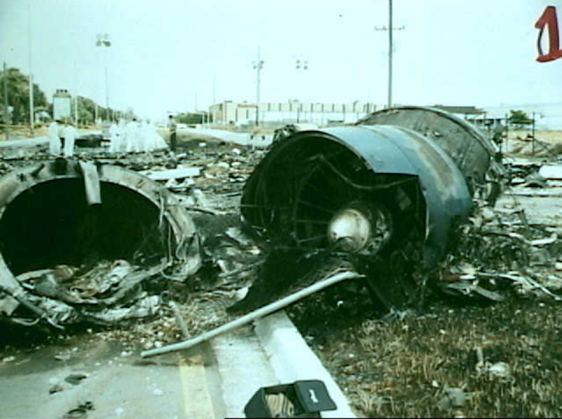
Powerplants 8. Photo 2. Number 1 Engine Front View
