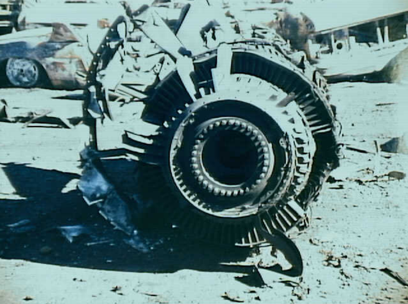
Powerplants 8 - Photo 8. Front view of No. 2 engine showing fan disk.
