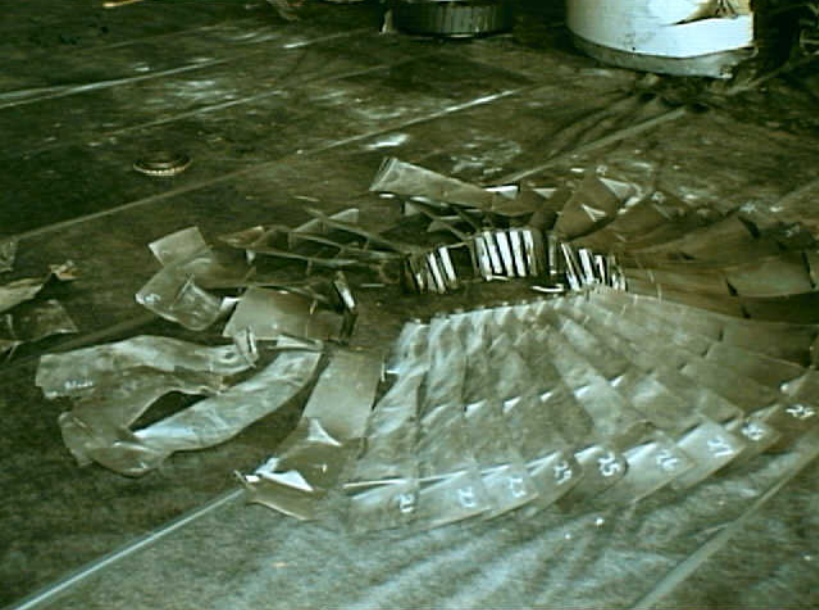
Powerplants 8 - Photo 7. Engine No. 1, fan blades
