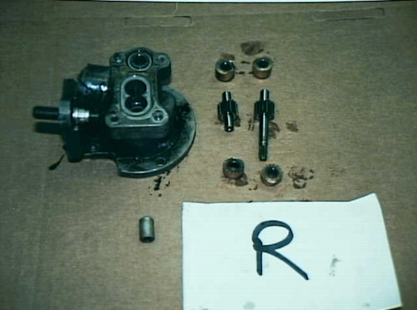
Powerplants 8 - Photo 64. Right auxiliary electric pump housing and gears
