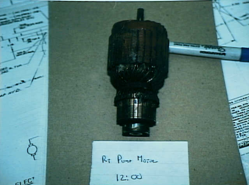
Powerplants 8 - Photo 62. Right auxiliary electric pump motor at 12:00 position
