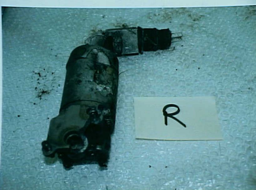
Powerplants 8 - Photo 61. Right auxiliary electric pump as received at AeroControlex
