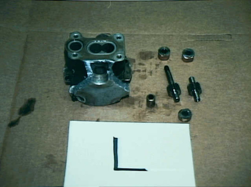
Powerplants 8 - Photo 60. Left auxiliary electric pump housing and gears
