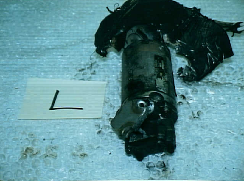
Powerplants 8 - Photo 57. Left auxiliary electric pump as received at AeroControlex
