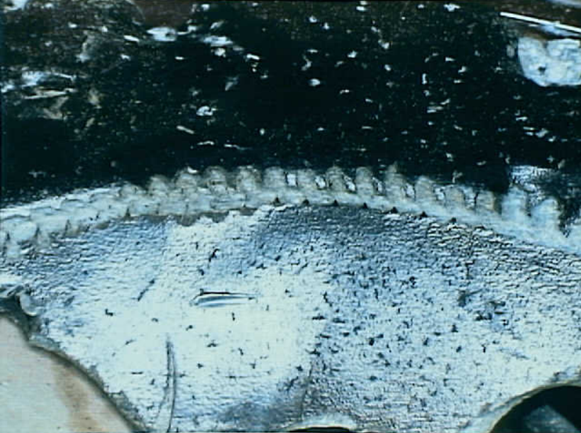
Powerplants 8 - Photo 56. Close up imprint of bull gear on right engine reduction gear box
