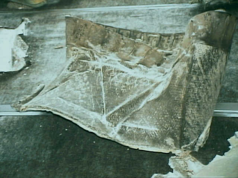
Powerplants 8 - Photo 52. Turbine exhaust plug segment.
