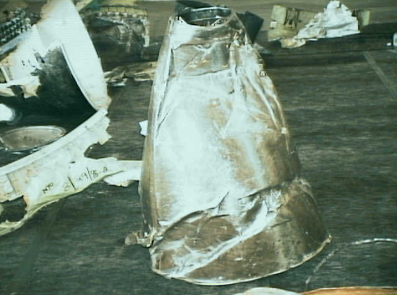
Powerplants 8 - Photo 51. Turbine exhaust plug segment.
