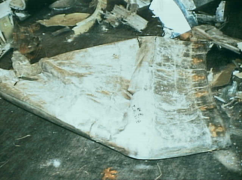
Powerplants 8 - Photo 50. Turbine exhaust plug segment.
