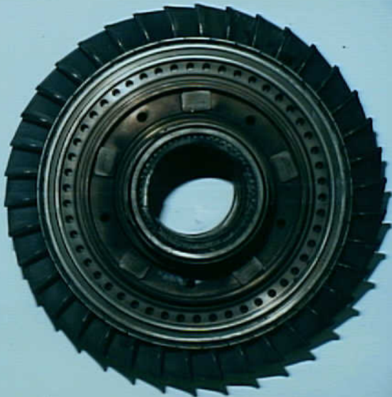
Powerplants 8 - Photo 50. Right engine high pressure turbine disk and blades
