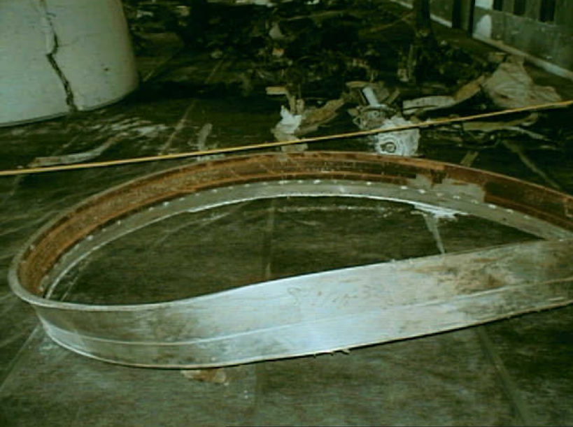
Powerplants 8 - Photo 5. Engine No. 1 fan rub strip, bottom.
