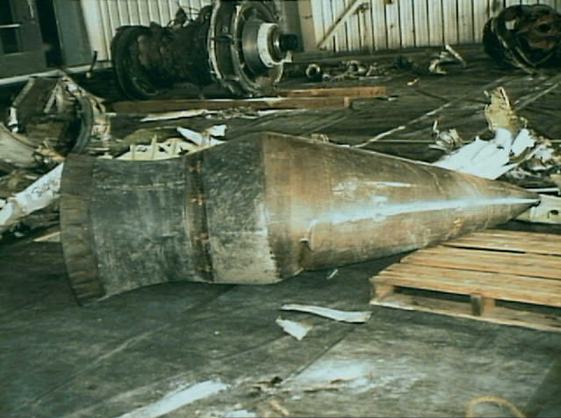
Powerplants 8 - Photo 49. Turbine exhaust plug.
