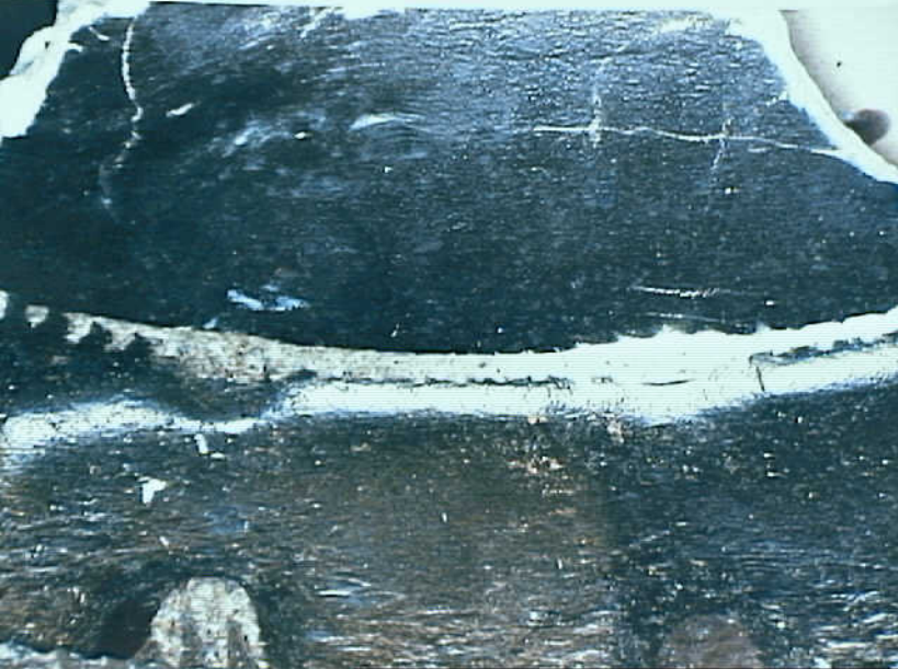
Powerplants 8 - Photo 44. Close up of left engine reduction gear box showing imprint of bull gear
