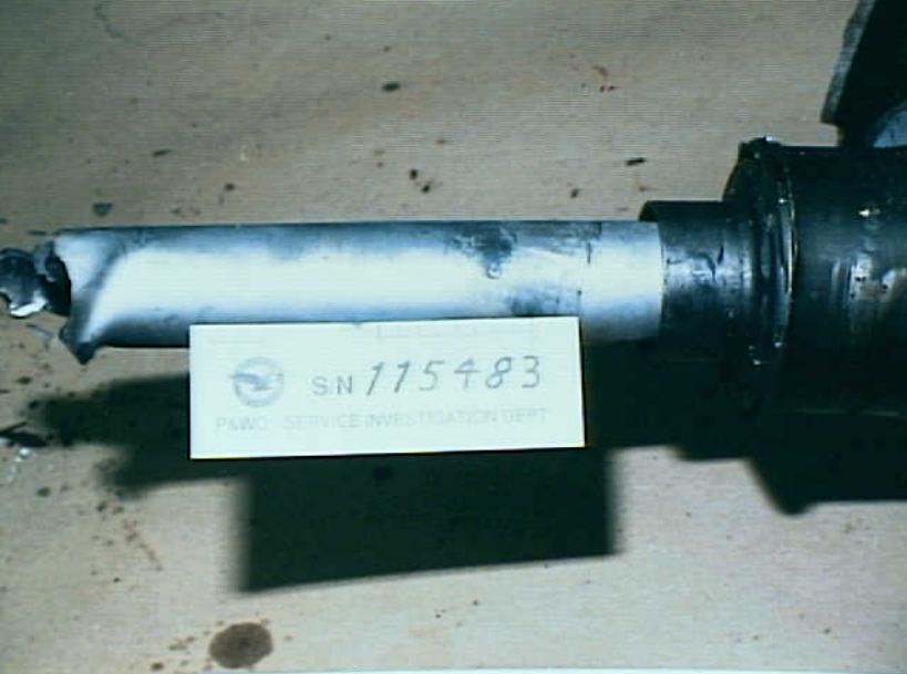
Powerplants 8 - Photo 43. Left engine propeller drive shaft
