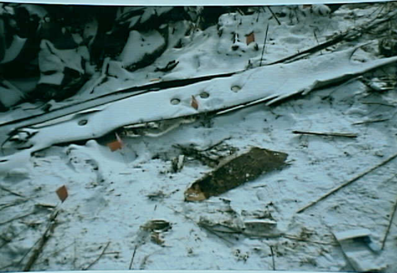
Powerplants 8 - Photo 4. Left propeller blade tip fiberglass shell and foam core
