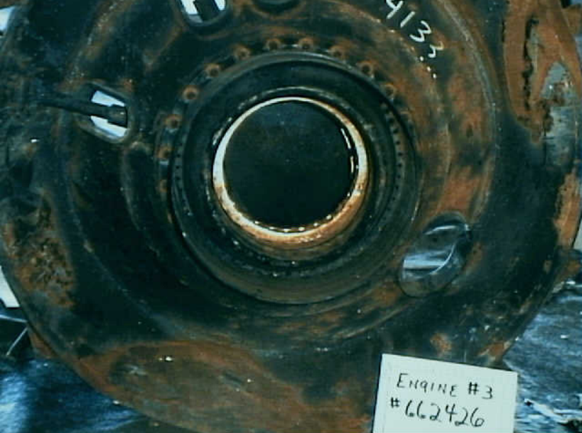
Powerplants 8 - Photo 38. Engine No. 3, No. 4, bearing, bearing housing, and support.
