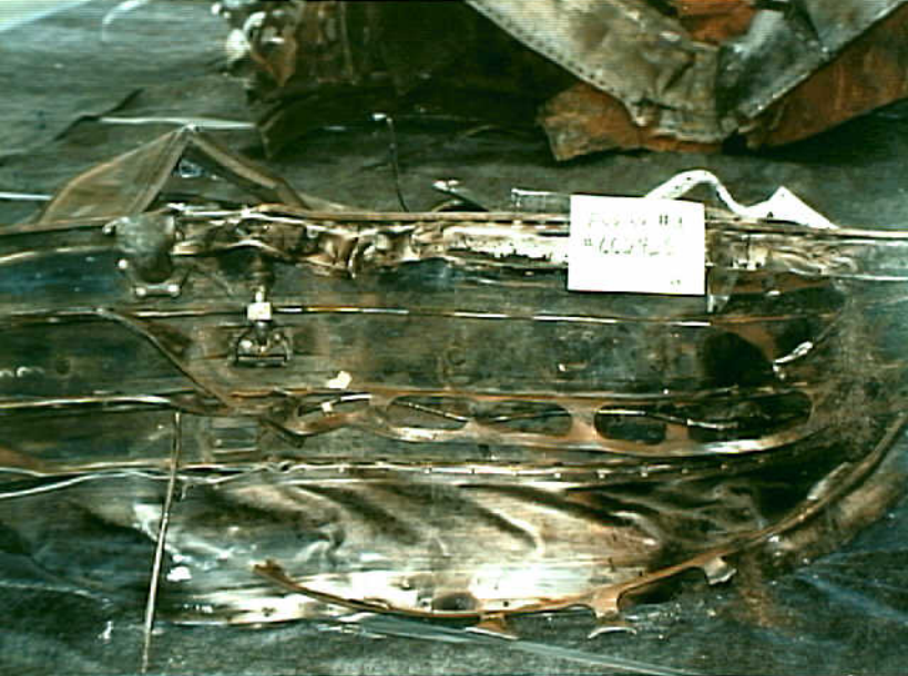
Powerplants 8 - Photo 36. Engine No. 3, turbine exhaust case.
