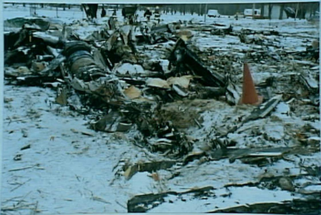
Powerplants 8 - Photo 3. Right engine and propeller at crash site
