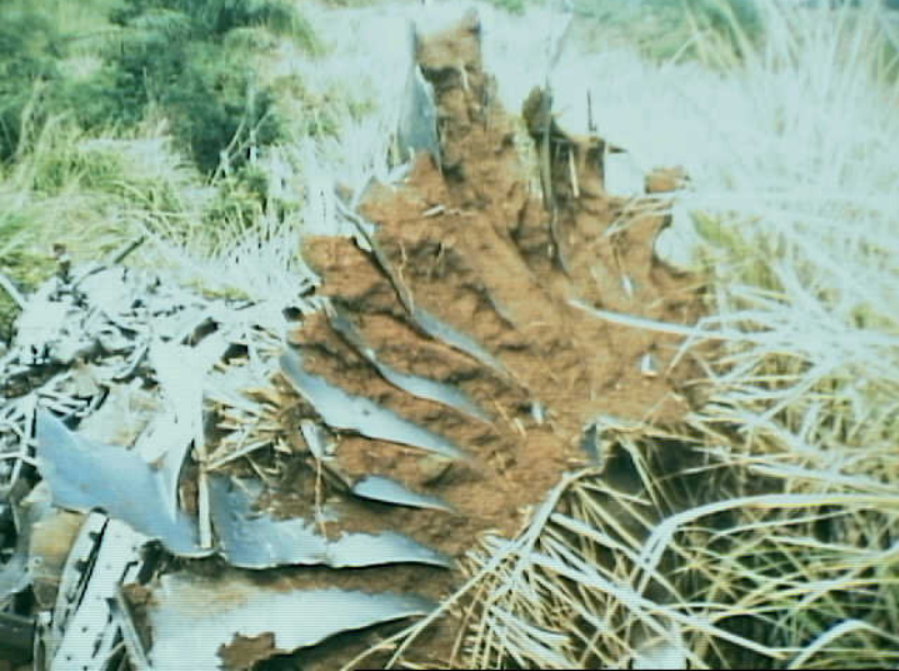
Powerplants 8 - Photo 3. No. 1 engine fan
