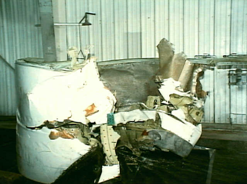
Powerplants 8 - Photo 3. Engine No. 1 inlet cowling, lower left side, and inlet duct.
