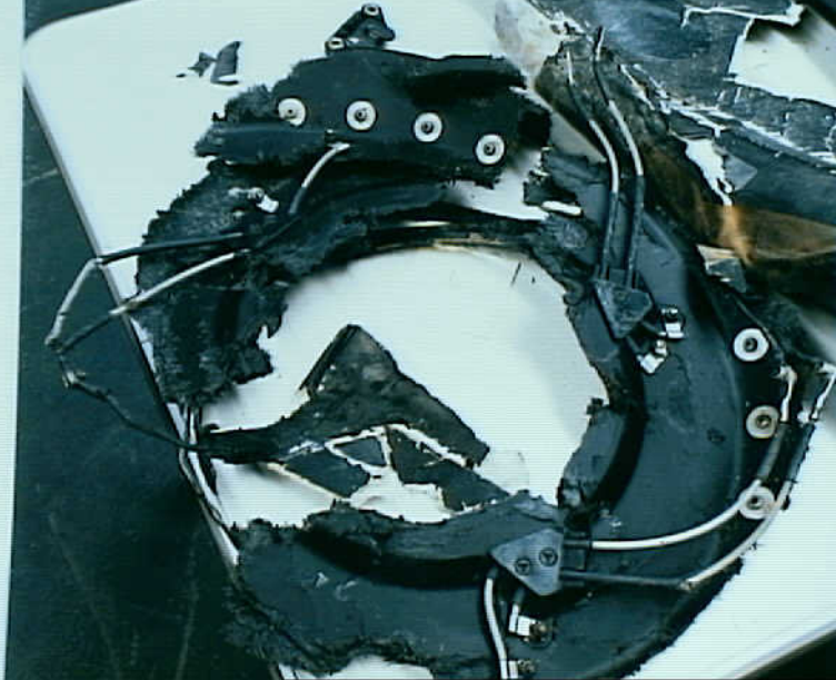
Powerplants 8 - Photo 28. Left propeller bulkhead and electrical leads
