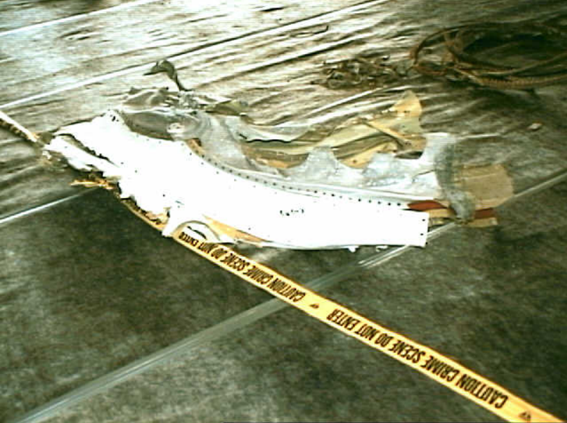
Powerplants 8 - Photo 27. Engine No. 3, piece of nacelle inlet.
